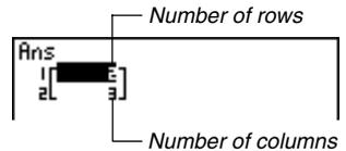
The display shows that Matrix A consists of two rows and three columns.
