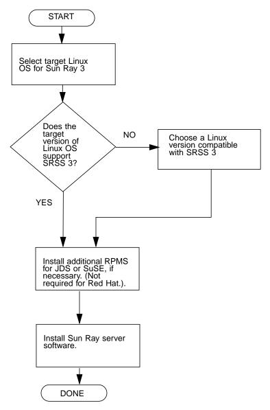
FIGURE 1-1 Installation Flow Chart
