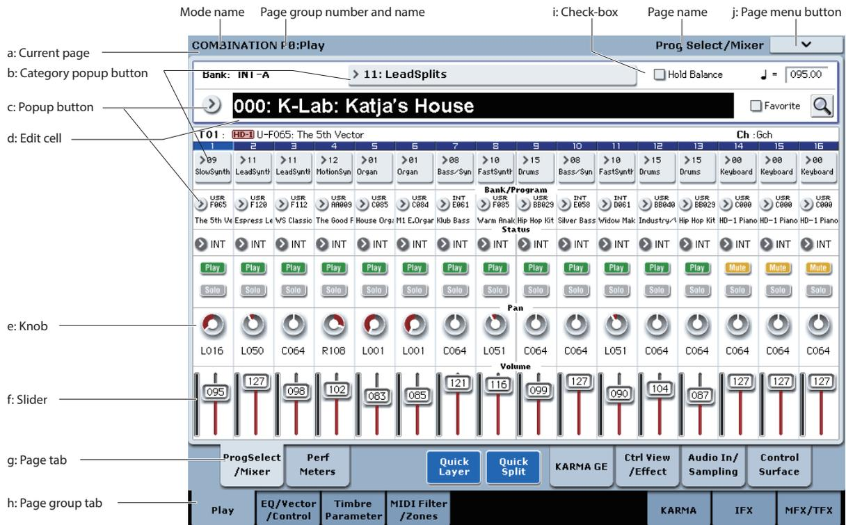
The KRONOS uses Korg's TouchView graphical user interface. By touching objects displayed in the LCD screen, you can select pages, set parameter values, move sliders and knobs, enter text, connect virtual patch cables, and more.
