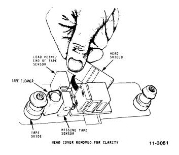
Figure C-3 TS03 Tape Head Assembly
