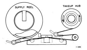
Figure 3-1 Tape Threading Diagram
