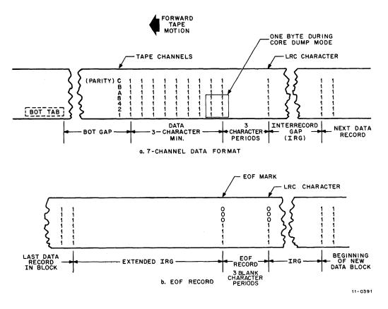
Figure A-5 7-Channel Tape Format
