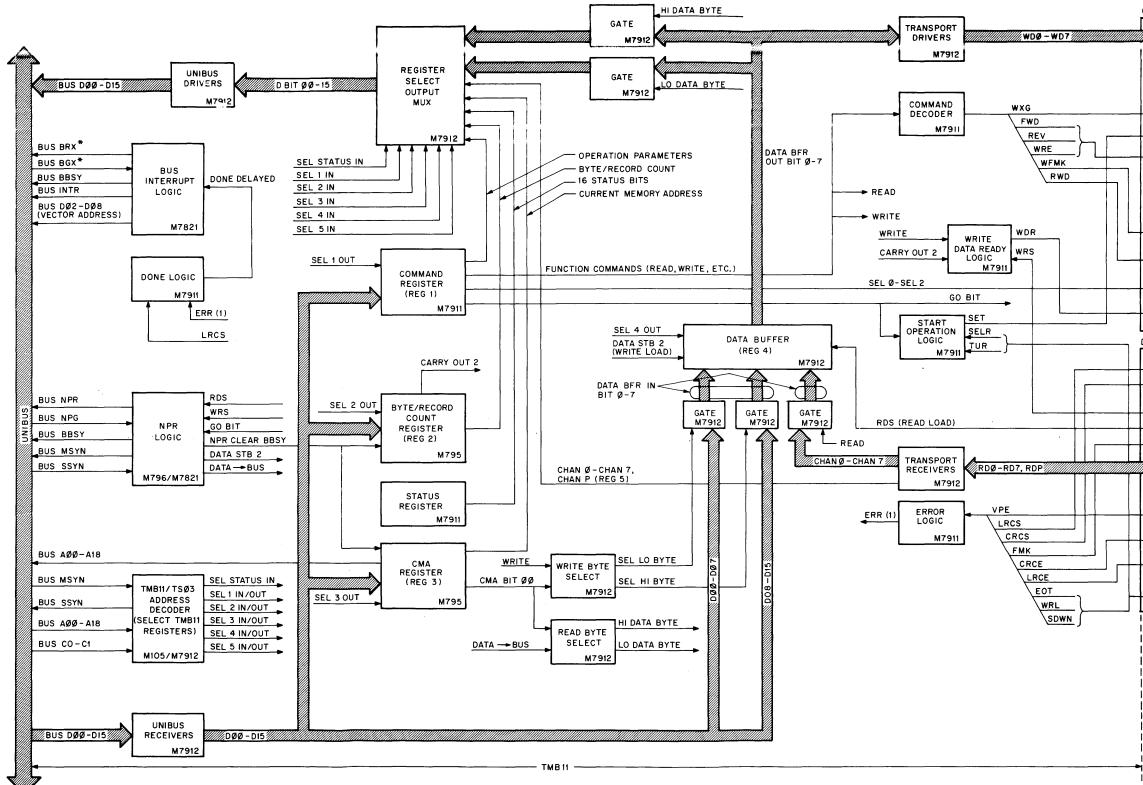
Figure 1-5 TMB11/TS03 Functional Block Diagram (Sheet 1 of 2)
