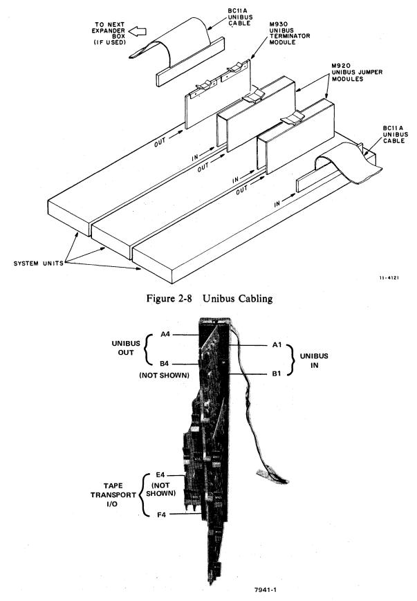
Figure 2-9 TMB11 Mounted in System Unit
