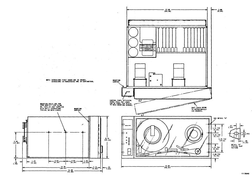
Figure 2-3 TS03 Transport Physical Dimensions
