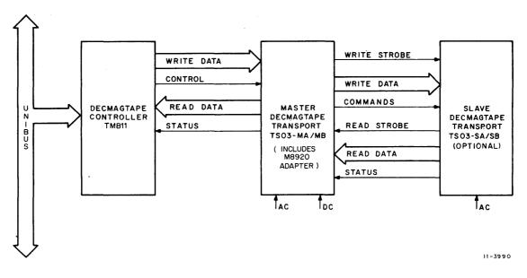
Figure 1-1 TMB11/TS03 System Configuration
