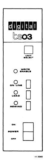
UNIT SELECT Plug – One of two plugs can be inserted, designating unit as 0 or 1.
