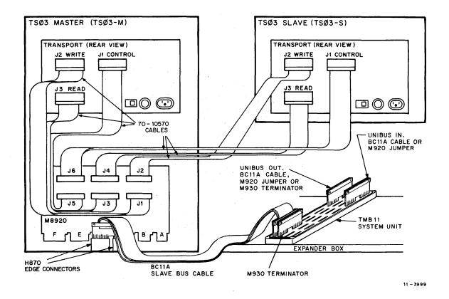
Figure 2-11 I/O Cable Connection Diagram
