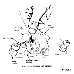
Figure 4-1 Opening Head Shield
