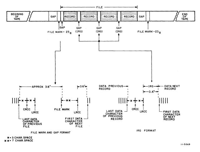
Figure A-3 Data Recording Scheme
