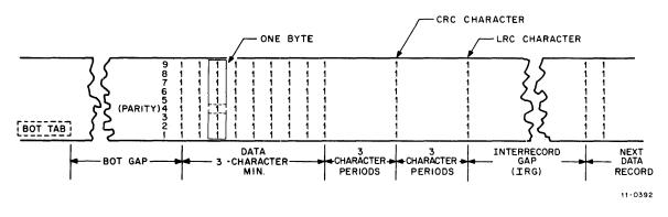
Figure A-6 9-Channel Tape Format
