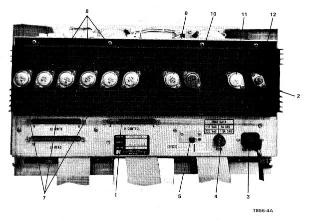
Figure B-3 Tape Transport Parts Identification (Rear View)
