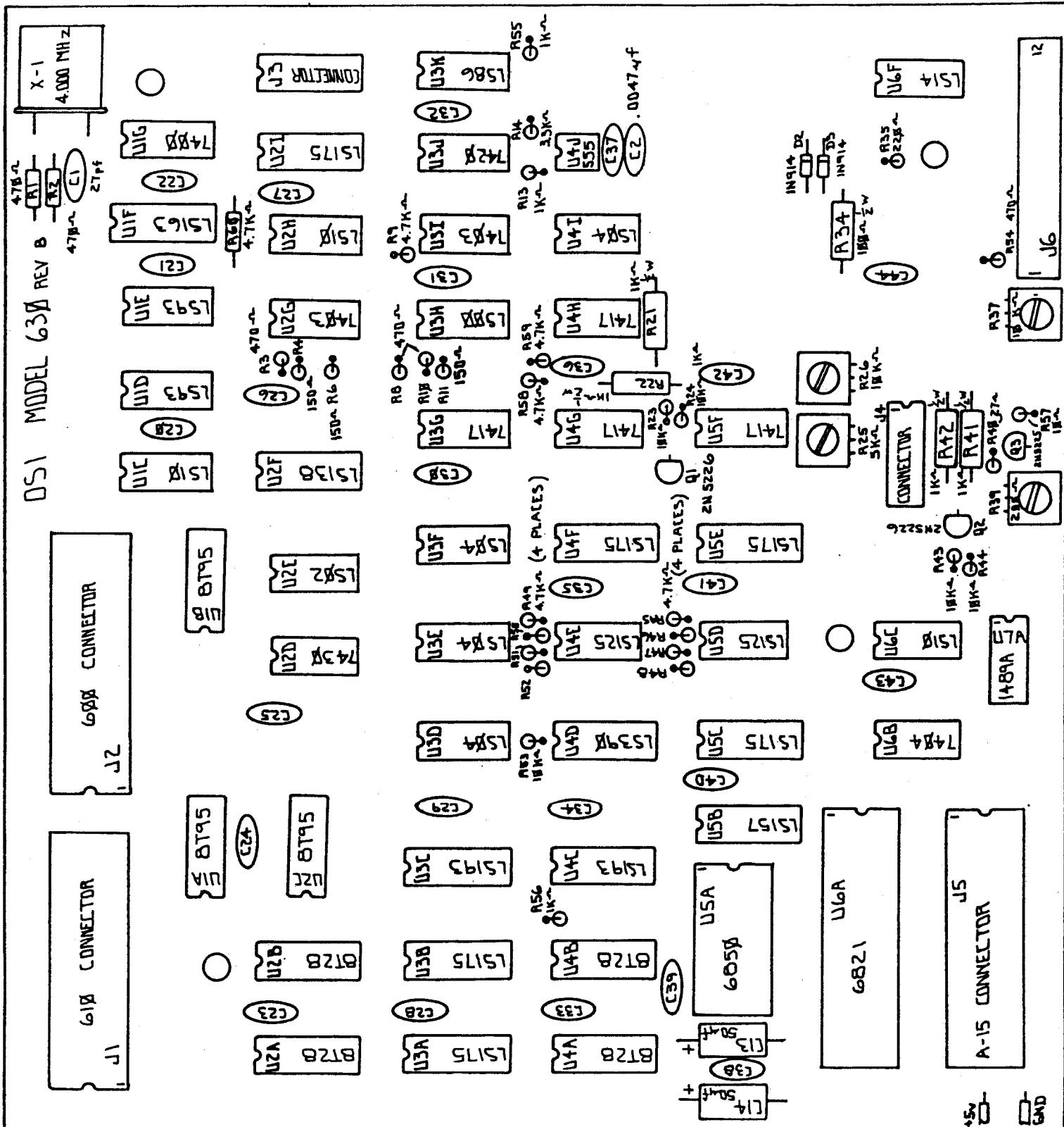
C20-C44 ARE .1uf BYPASS CAPACITORS
