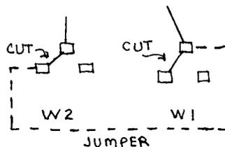
This converts Pin 21 on the 2716 EPROM from 02 clock to +5 volts. I suspect a similar change is required on BASIC 3 as well. Until I made these changes, my C1 required a "warm-up" period of 5 to 10 minutes. Now, it "boots up" at once.
