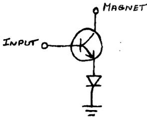
Since TTL gates can only source about .8 ma in the high state, Darlington transistors are required. I used GE type D40C4 rated at 6 watts, 0.5 amps, 40 volts, with a gain of 10,000. The diode is a 1 amp 50 piv rectifier. It serves to protect the transistor from the counter emf generated by the magnet coil. Note - for 48 volt magnets, use a D42D3 transistor with a 1 amp 100 piv diode.
