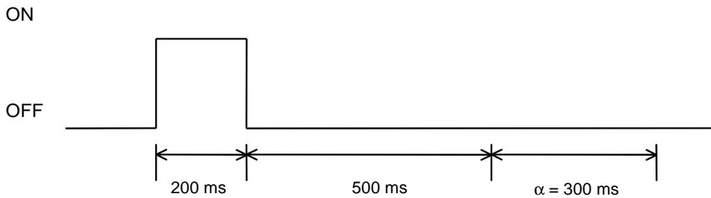
**Figure D-2 Drawer Drive Signal Waveform**
