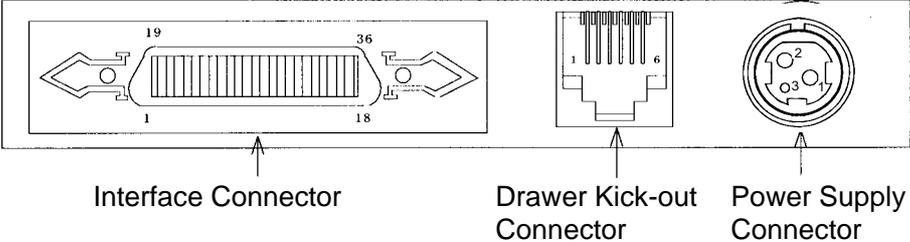
**Figure 2.2.2 Parallel Connector Panel Diagram**
