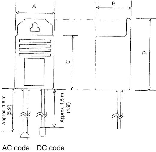
**Figure 5.1.1 External Appearance of the AC adapter**
