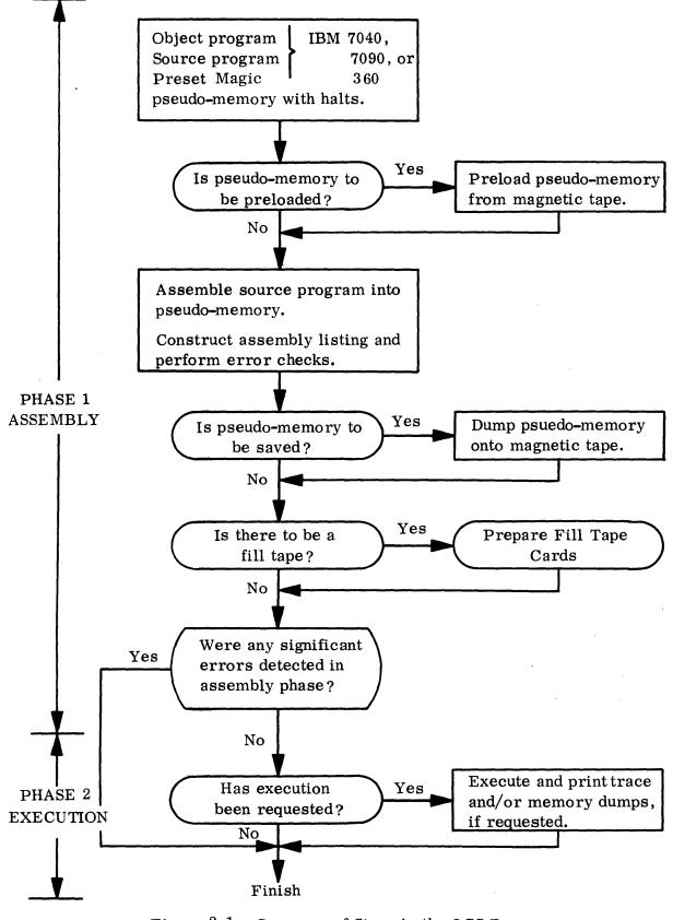
Figure 2-1. Sequence of Steps in the OCS Process
