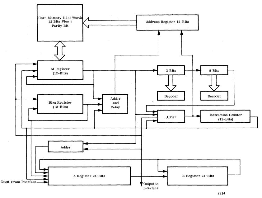
Figure 3-1. Central Processing Unit Block Diagram
