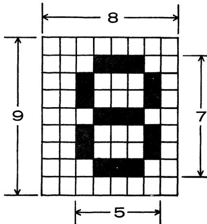
To generate a character on the screen the Read Only Memory, ROM, must supply seven five-bit words to the video shift register, one for each of the seven scan lines used to display the character. During each scan line at the given character position the video shift register shifts the five bits to the video mixer at the 12.528 MHz rate. These bits make the video black for ones and white for zeroes, assuming a normal black on white presentation.
