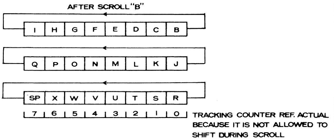
line where they should be. The same is true of memories #1 and #2. In order to correct this situation, the Tracking Counter must be allowed to go out of sync for the 80 shifts. This is done by not allowing it to count during the time the memories scroll. This reassigns the lines such that the spaces are in line 7. The bottom of Figure 2.8 shows the actual relationship between the data and the Tracking Counter. Note the Tracking Counter hasn't changed from the top reference.
