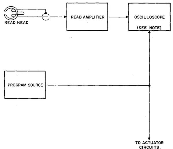
NOTE: ADJUST SCOPE TO TRIGGER ON POSITIVE INPUT TO MEASURE START TIME, ON NEGATIVE INPUT TO MEASURE STOP TIME.
