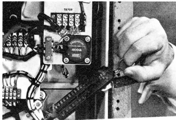
Step 2: Remove the blower wiring at TB708 (located inside the end cap).
