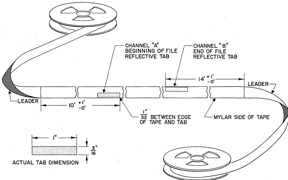
Figure 3-5. Placement of Photosense Tabs on Tape
