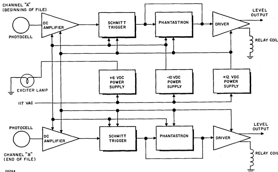
Figure 6-13. Block Diagram, Photosense Electronics
