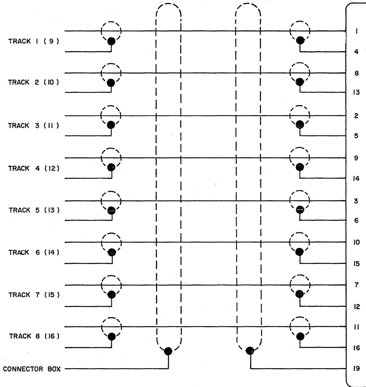
Figure 2-8. Head Cable Connections
