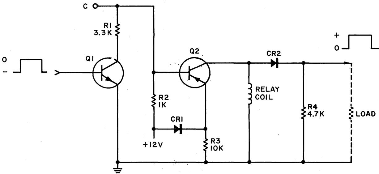
Figure 6-16. Photosense Output Circuit
