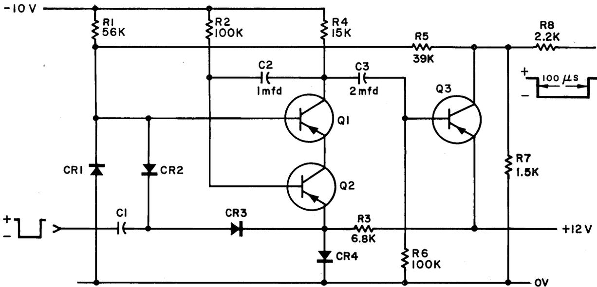
Figure 6-18. Photosense Phantastron Circuit
