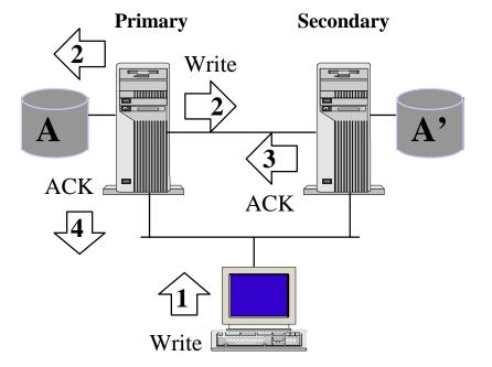
Figure 2: Shared Nothing Configuration—Server Initiated Copy to Secondary
