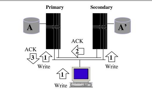
Figure 3: Shared Nothing Configuration—Network-based Data Replication
