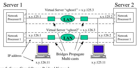
Figure 5: ServerGuard Over a Bridged Network
