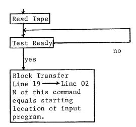
This is called a "loader" program. Its value is derived from the fact that, if p is used to cause the reading of a block of tape, and if, after the input has ceased, the enable switch is turned off and the compute switch is turned to GO, the computer will take its next command from 23.00, which, as you know, will be the same as 19.00. Now we can trace the operation of this program.
