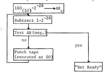
In the program flow-diagrammed on the preceding page, N in the punch tape command will equal the word-time in which the subtract command is located. The program will continue looping and counting the elapsed drum cycles by subtracting 1 from 180 for each drum cycle. Eventually AR will contain +0, and when 1 is subtracted from it, it will contain -1, the answer to the test will be "yes", and the program will exit from the loop. At this point the proper length of blank tape will have been punched.
