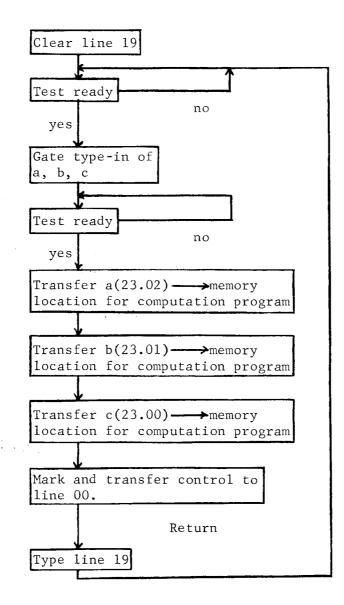
In addition, we must include a command at the end of the program in line 00, a mark and transfer control command, which will transfer control back to this program at the correct point, for the type-out of the answers.
