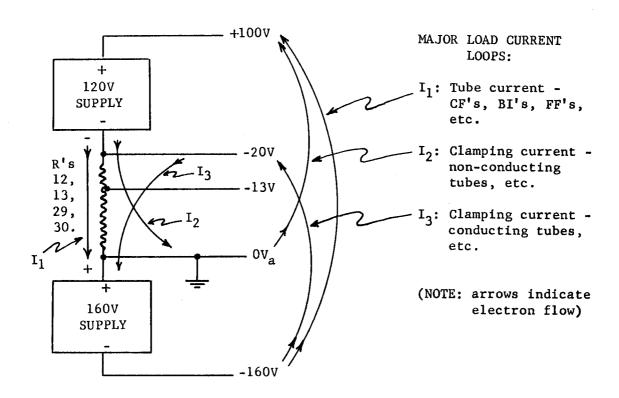
G-1c This hookup yields four stable output voltages by means of only two supplies. Drawing 58 shows the details of the arrangement.
