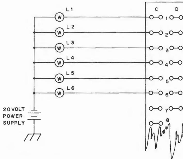
Figure 20. Internal Wiring for Rows C and D
