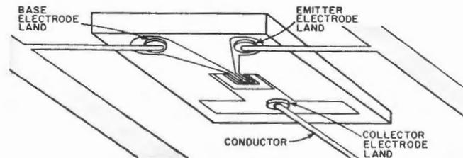
FIGURE 7 - Construction of a transistor of the flip-chip form.
