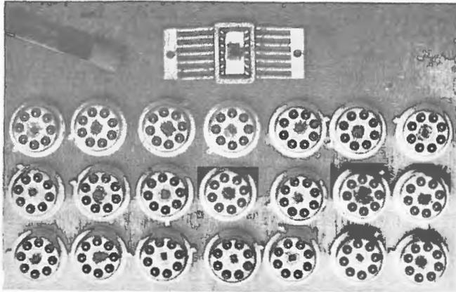
FIGURE 3 - A 21-bit register (top) whose heart is a microscopic wafer of silicon containing 110 transistors and 48 resistors, replaces 21 separate microcircuits (shown here) in computers.
