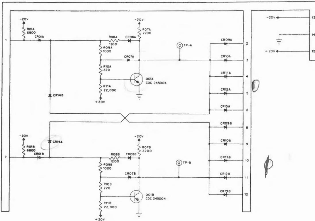
Figure 75. Standard Flip-Flop
