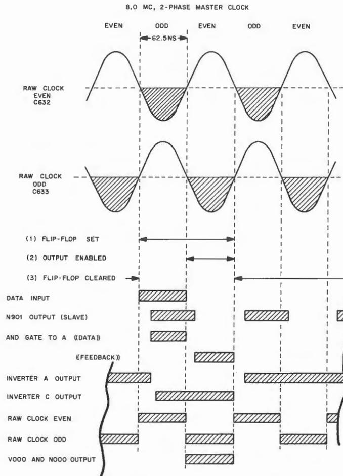
Figure 105. Control Delay Timing
