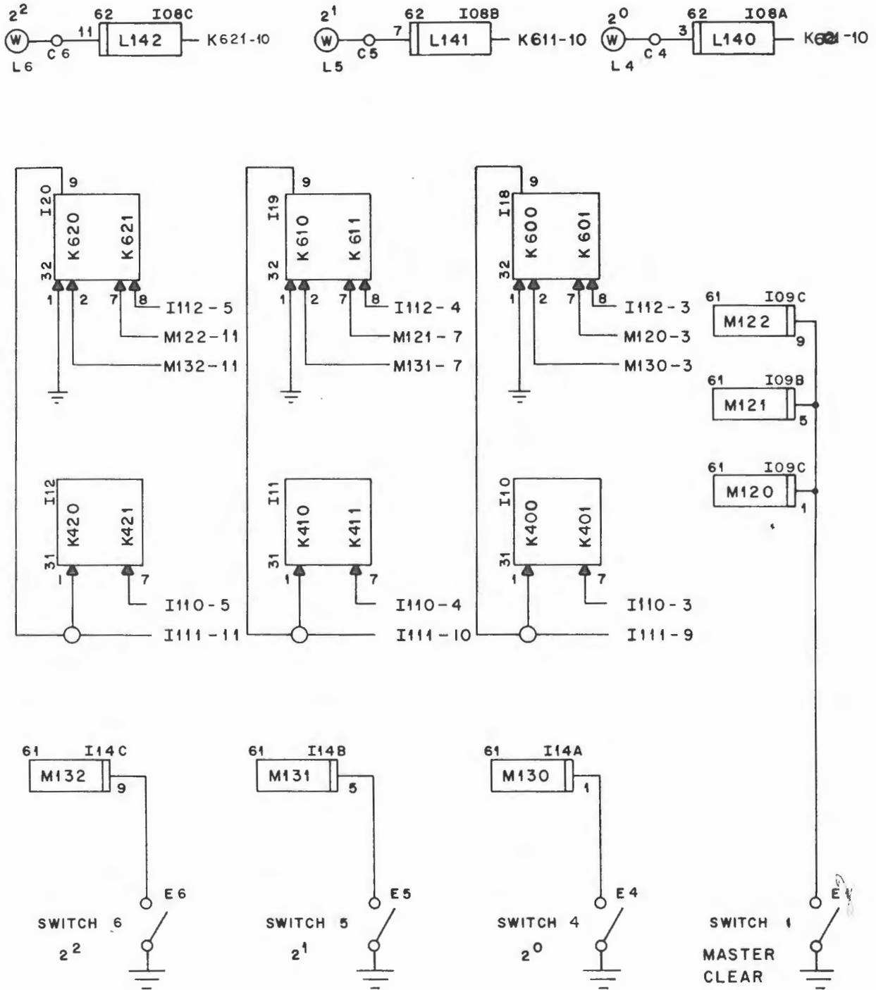
Figure 48. Three-Stage, Double-Rank Register
