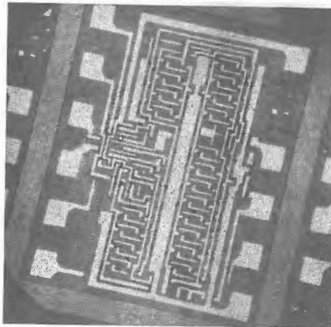
FIGURE 4 - A 21-bit shift register. The functional block diagram and a photomicrograph of the actual structure used.
