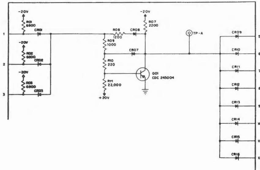
Figure 68. Three-Input Inverter
