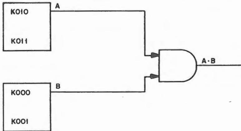
Figure 124. AND Gate Decoder
