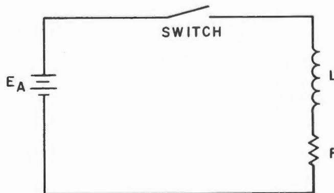
Figure 88. Basic RL Circuit
