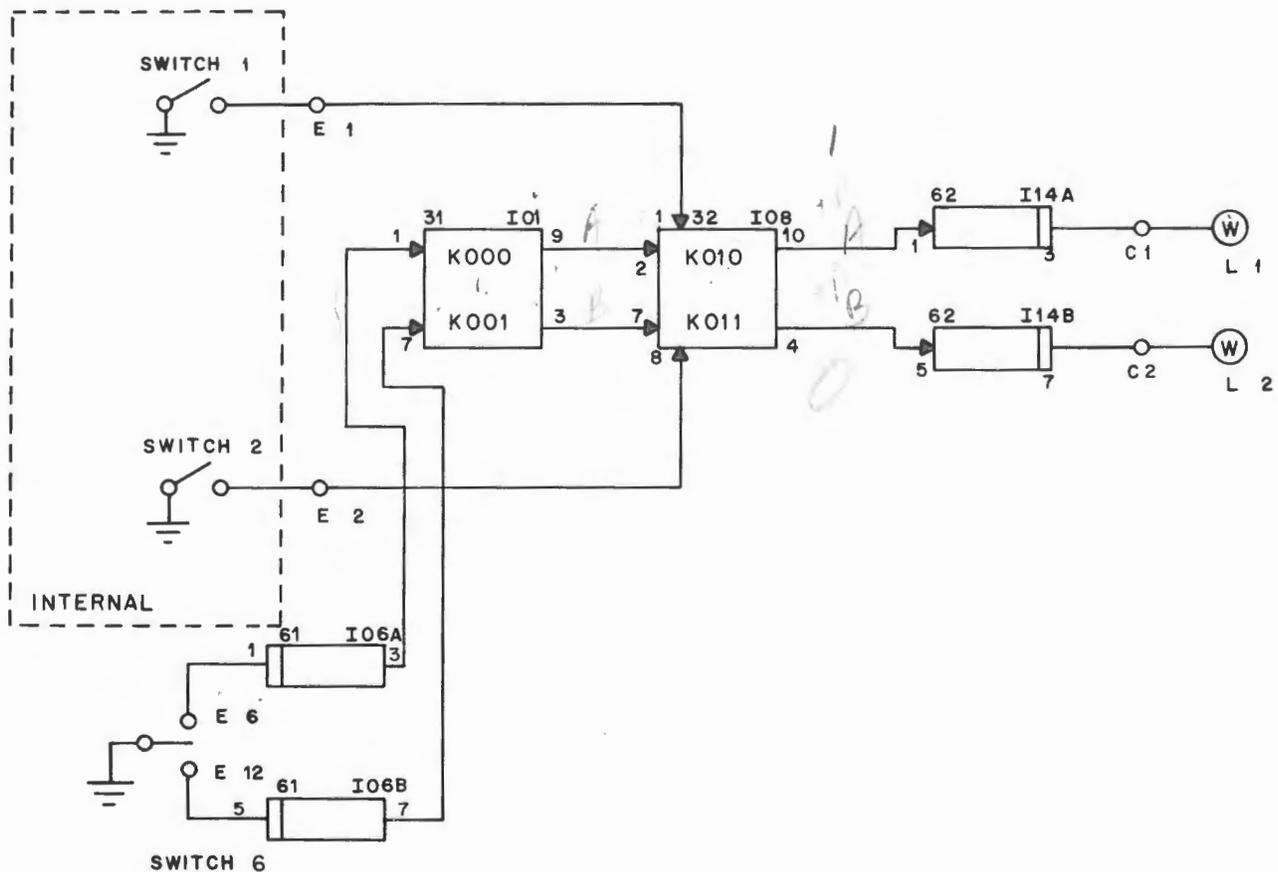
Figure 34. Flip-Flop as Gate Circuit
