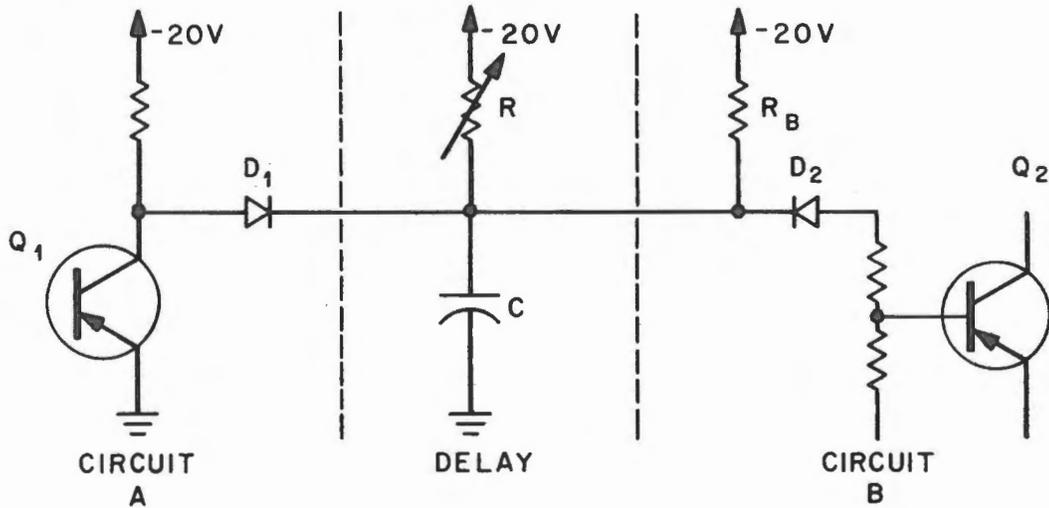
Figure 91. Capacitive Delay
