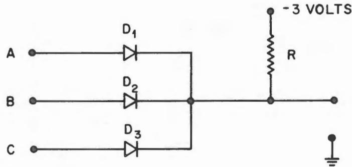
Figure 56. Diode AND Gate Negative Logic
