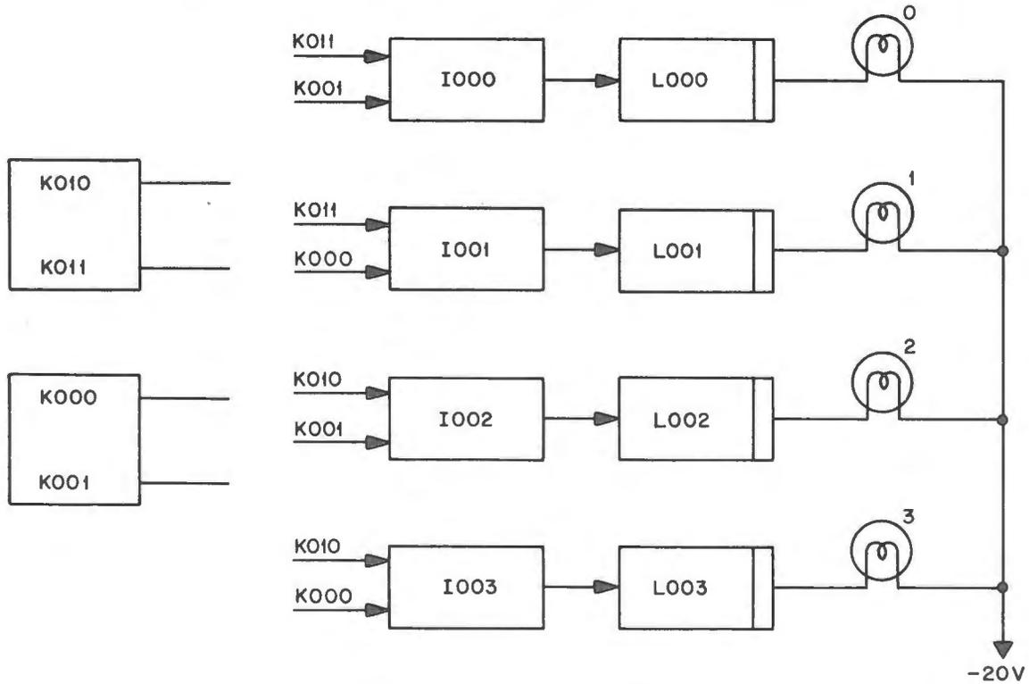
Figure 128. Four-Stage Inverter Decoder
