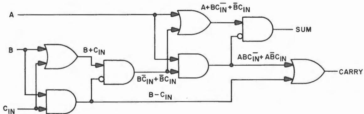
Figure 121. Full-Adder Logic Diagram
