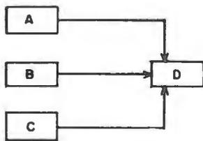
Figure 70. Three-Input OR Circuit
