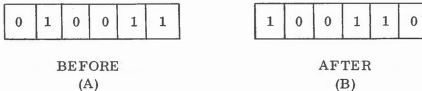
Figure 115. Left Shift, Zero End-Around
