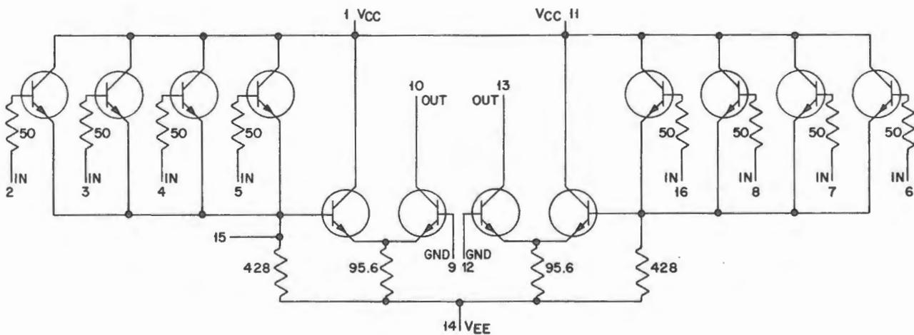
FIGURE 6 - Photo and schematic of hybrid 4-input gate.
