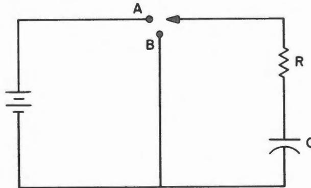
Figure 90. Basic RC Circuit
