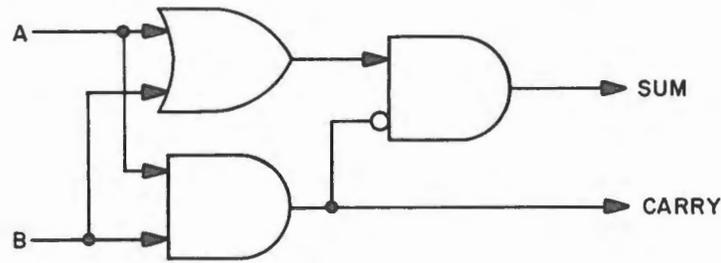
Figure 120. Half-Adder Logic Diagram
