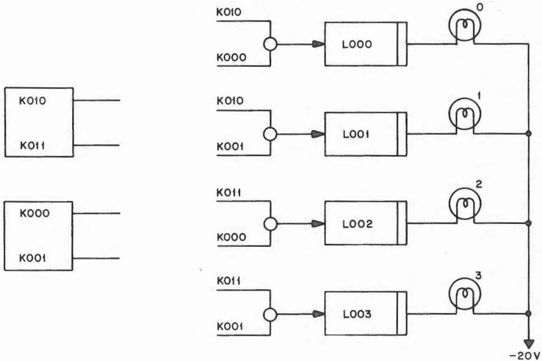
Figure 126. Four-Stage Decoder
