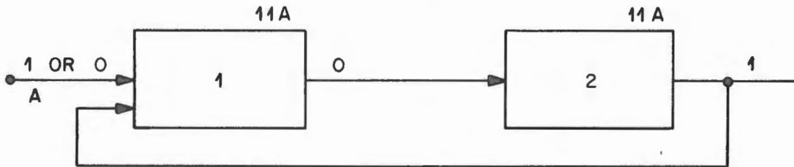
Figure 73. Two Inverters with Feedback
