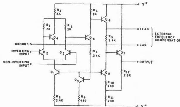
FIGURE 8 - An example of an integrated operational amplifier.
