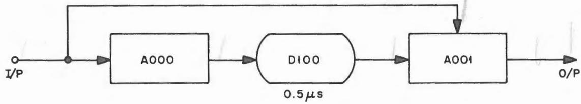
Figure 8. Pulse-Forming Network
