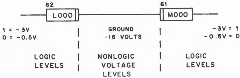
Figure 80. L and M Card Operation
