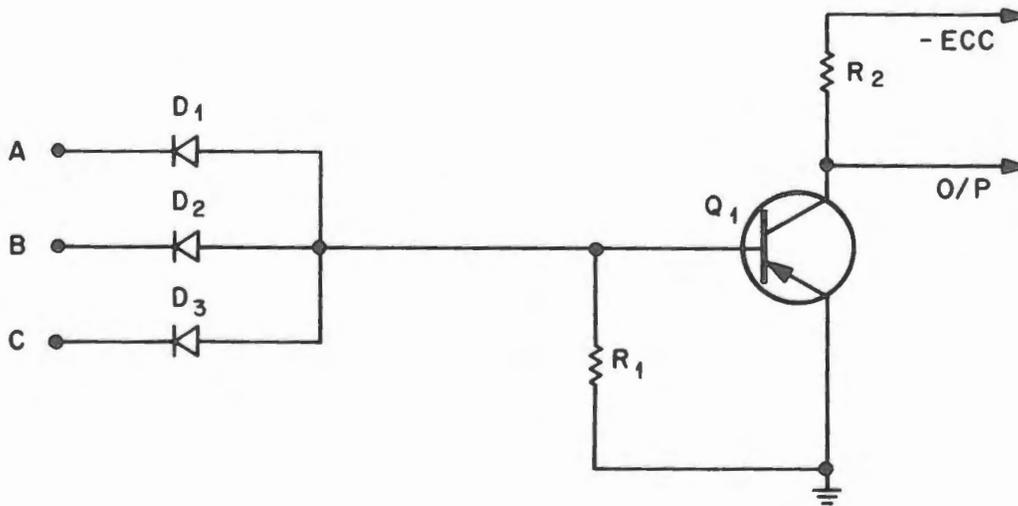
Figure 64. Diode/Transistor NOR Gate
