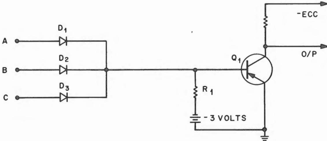
Figure 62. Diode/Transistor NAND Gate
