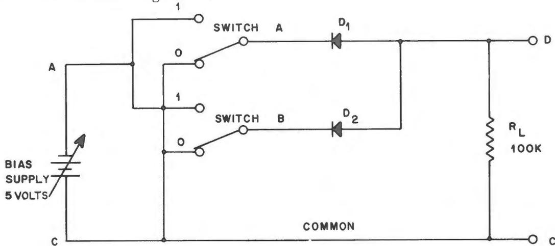
Figure 15. Diode OR Gate
