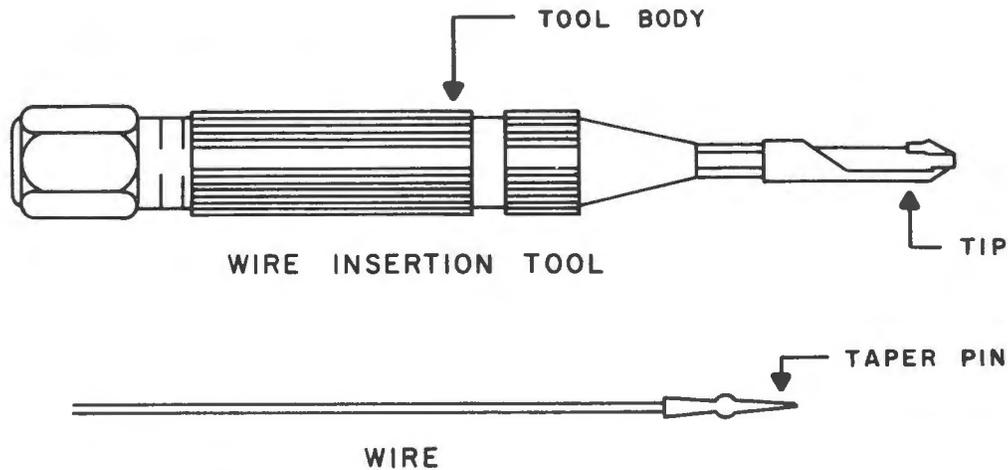
Figure 25. Wire Insertion Tool and Wire
