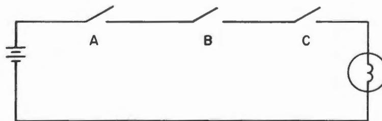
Figure 54. AND Circuit
