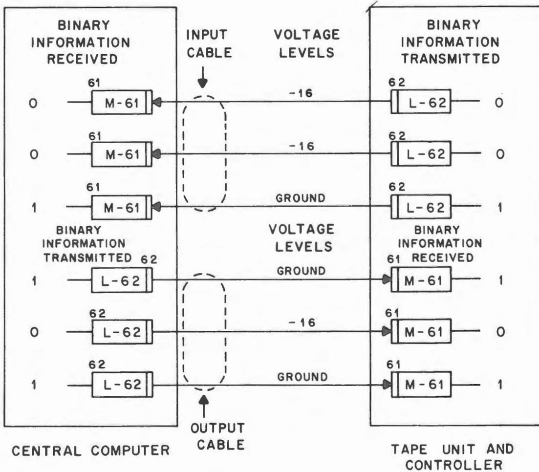
Figure 81. Transmission Lines
