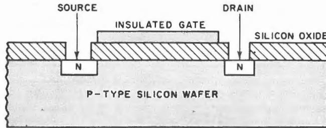
FIGURE 5 - Cross-sectional view of an "n"-channel MOS device.
