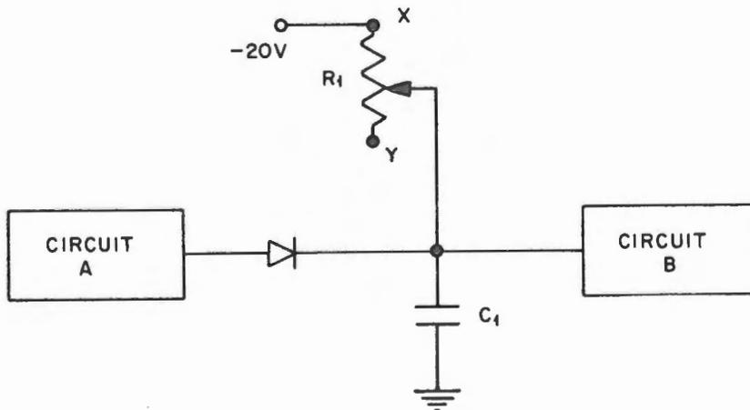
Figure 6. Determining the Amount of Delay
