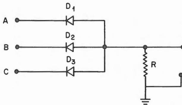
Figure 60. Diode OR Gate Negative Logic
