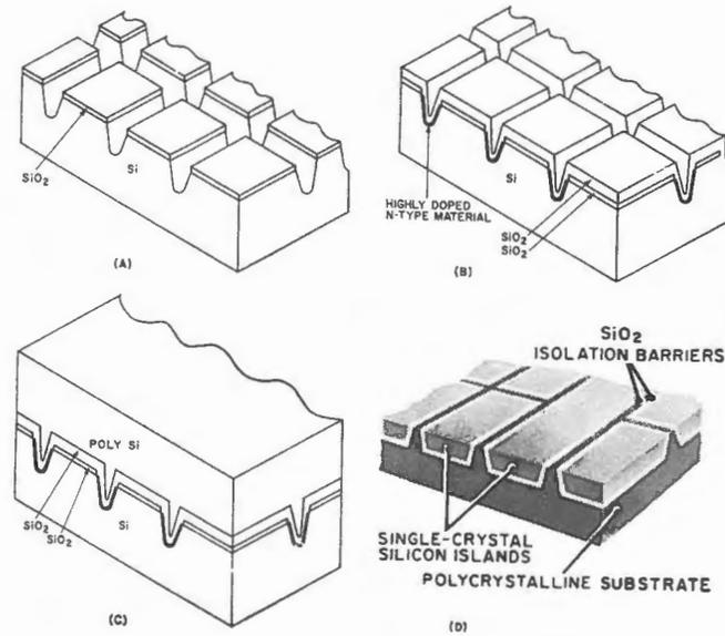
**FIGURE 1 - Isolated Monolithic Process**
