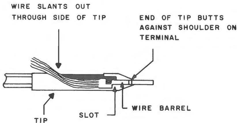
Figure 26. Cutaway View with Wire
