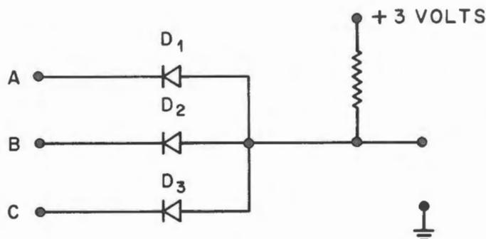
Figure 57. Diode AND Gate Positive Logic
