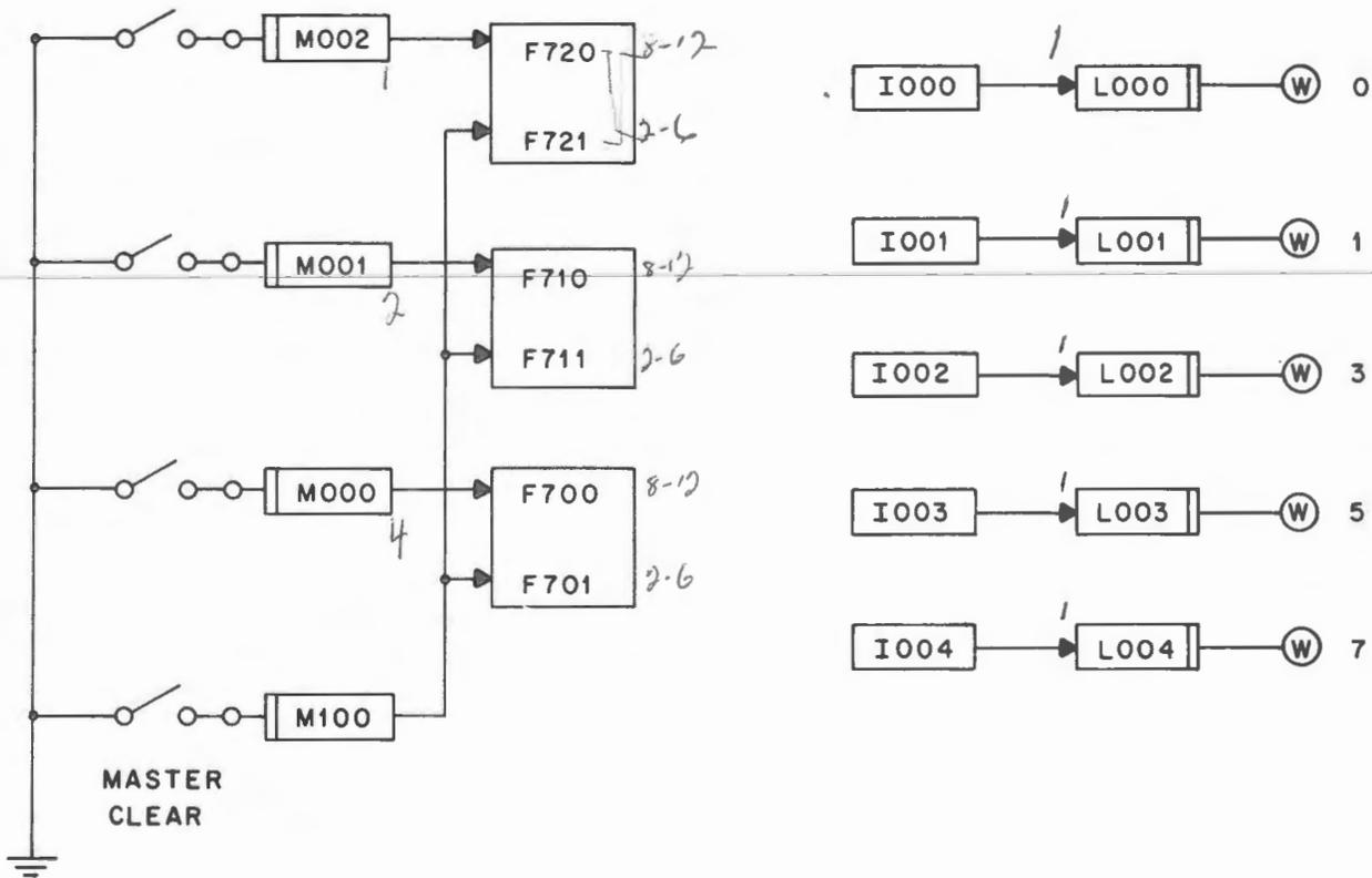
Figure 53. Translation and Decoding Network
