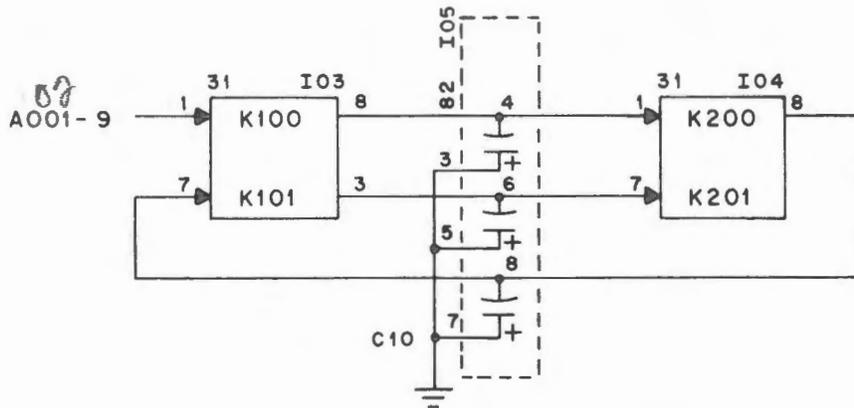
Figure 46. Timing-Chain Pulse Generator
