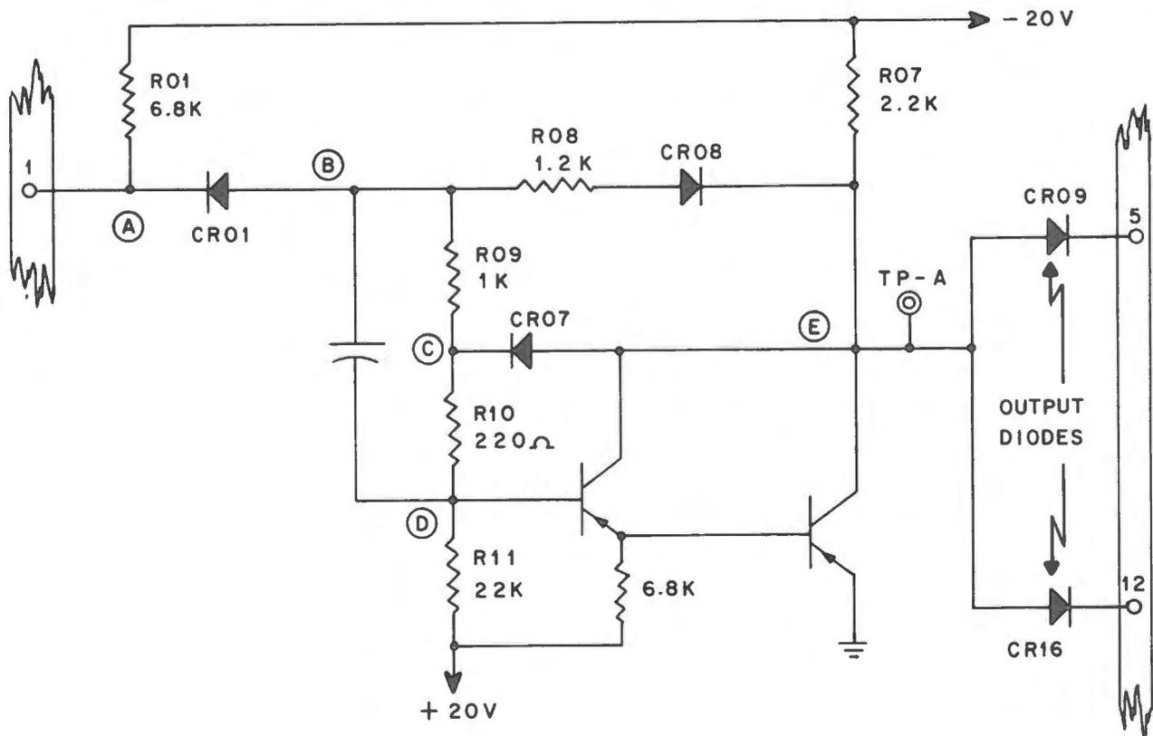
Figure 28. Single Inverter Circuit 11 Card
