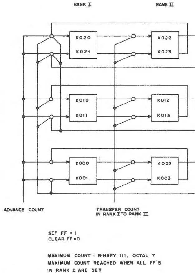
Figure 109. Three-Stage, Double-Rank Counter
