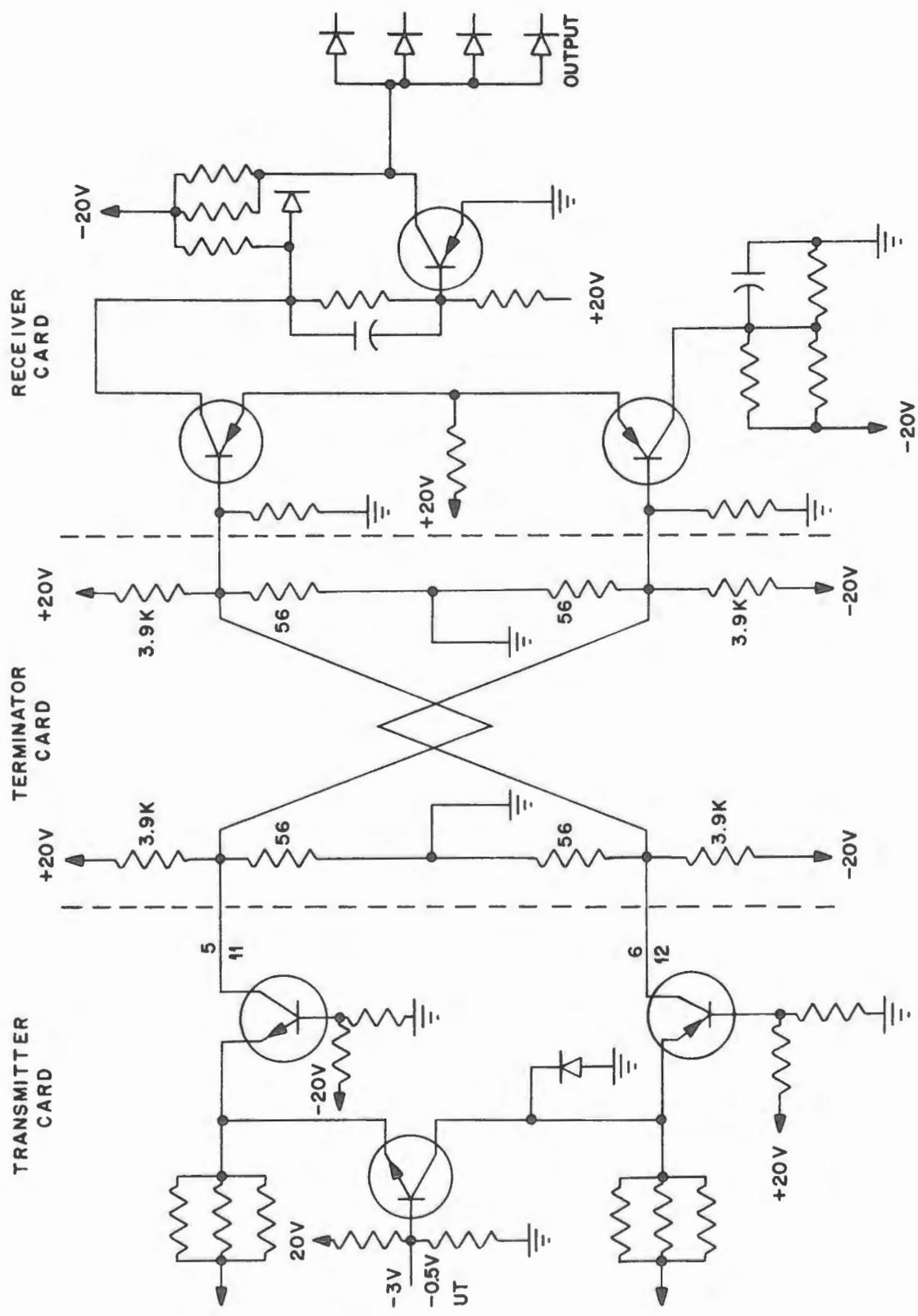
Figure 86. Transmitter/Receiver Circuit
