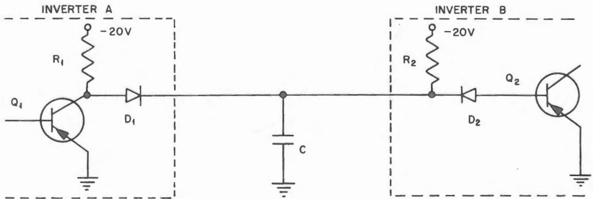
Figure 5. Delay Capacitor Charge Path
