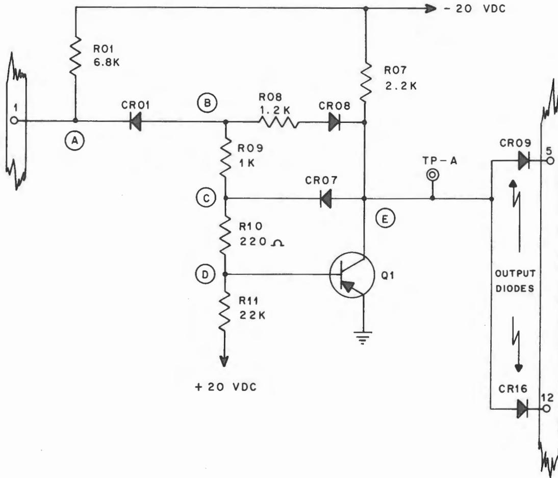
Figure 27. Single Inverter Circuit 11A Card
