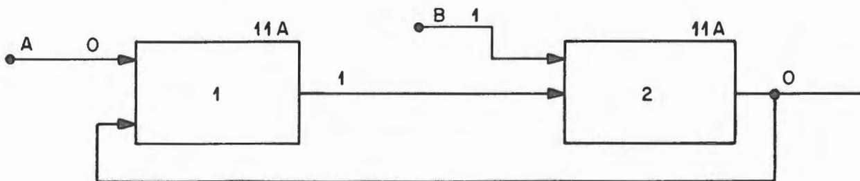
Figure 74. Basic Flip-Flop
