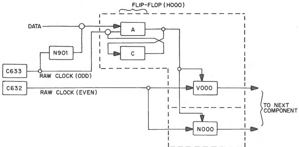
Figure 104. Even Control Delay
