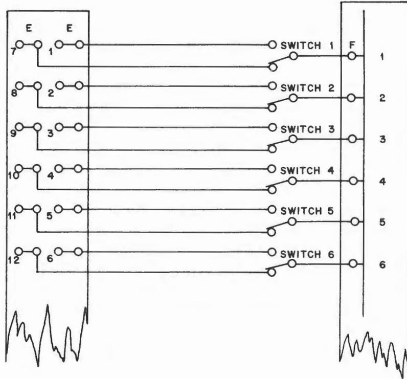
Figure 21. Internal Connections for Rows E and F
