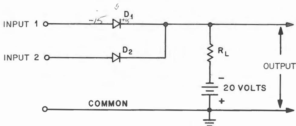
Figure 1. Identifying Diode States
