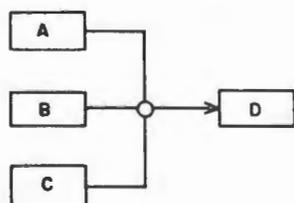
Figure 69. Three-Input AND Circuit
