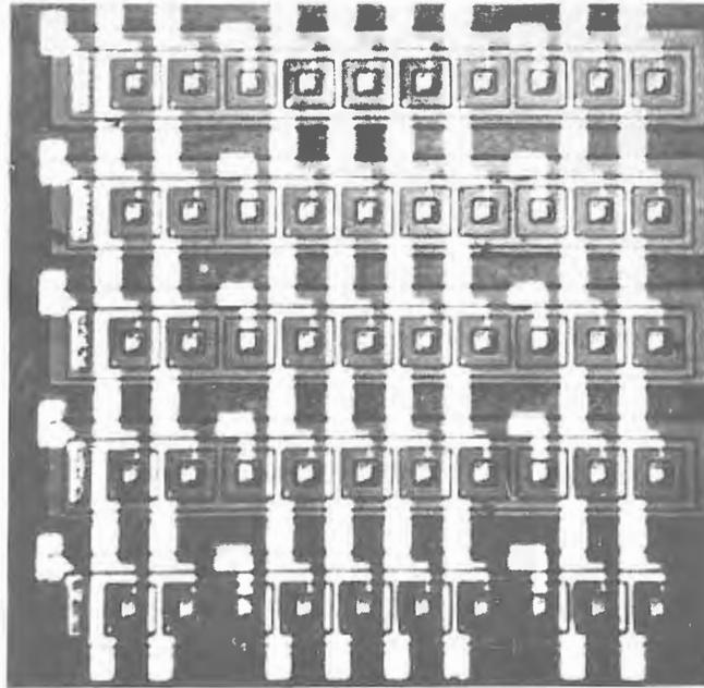
FIGURE 2 - Diode matrix made with isolated monolithic process.
