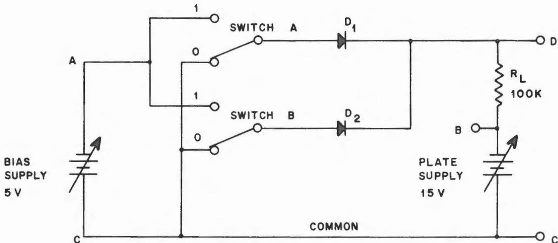
Figure 14. Diode AND Gate
