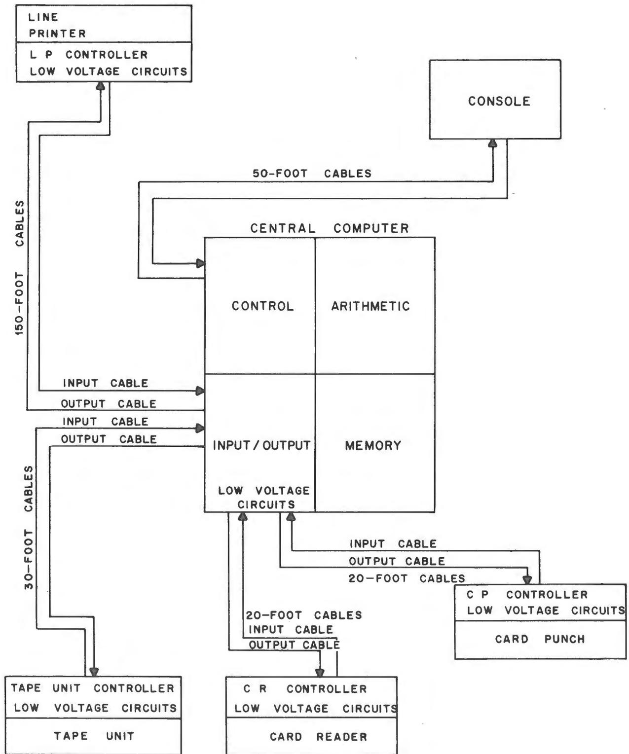
Figure 79. Computer System Block Diagram
