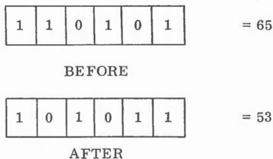
Figure 116. Left Shift, One End-Around
