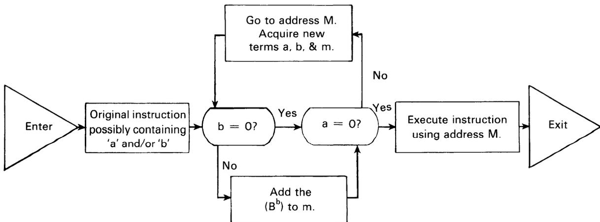
Figure 7-3. Indexing and Indirect Addressing Routine Flow Chart
