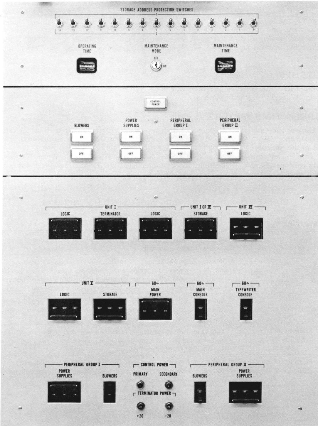
Figure 5-9. Power Control Panel
