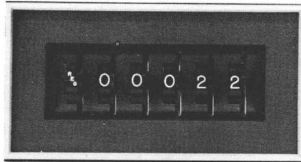
If the READ STO switch on the keyboard is depressed, the contents of register 22 are displayed in the Communication register at a repetition rate determined by the Auto Step control. (Only the lower two digits are of consequence when the REG designator is displayed. In this case register 22, the real time clock, is being referenced.)
