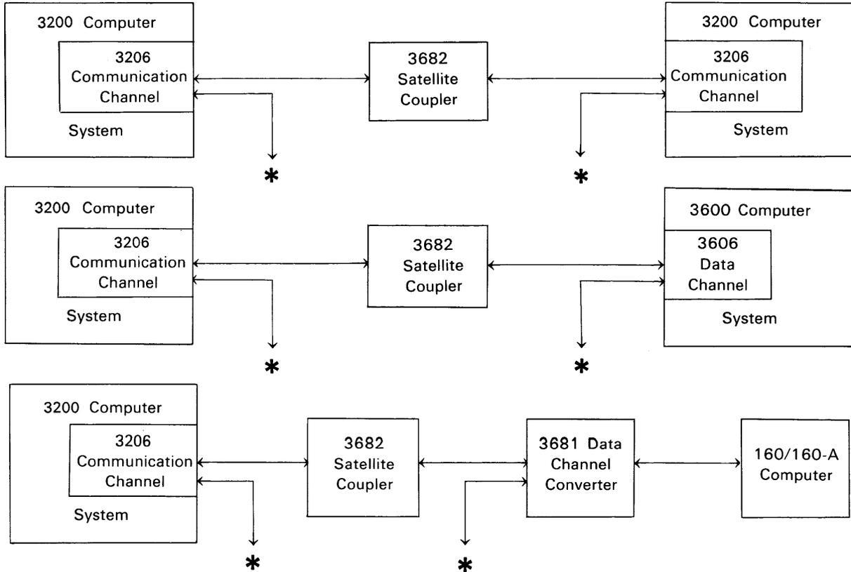
Figure 3-2. Satellite Configurations
