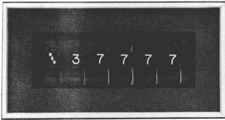
If the WRITE STO switch on the keyboard is depressed and data has been entered into the Communication register, the data will be transferred to register 77 when the TRANSFER switch is depressed. (Only the lower two digits are recognized when the designator switch is in the REG position. The programmer must use caution when writing into the Register File to prevent destruction of other data. Refer to Section 1, Table 1-3.)
