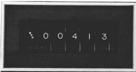
The computer stops only when an attempt is made to read or store an operand at address 00413.
