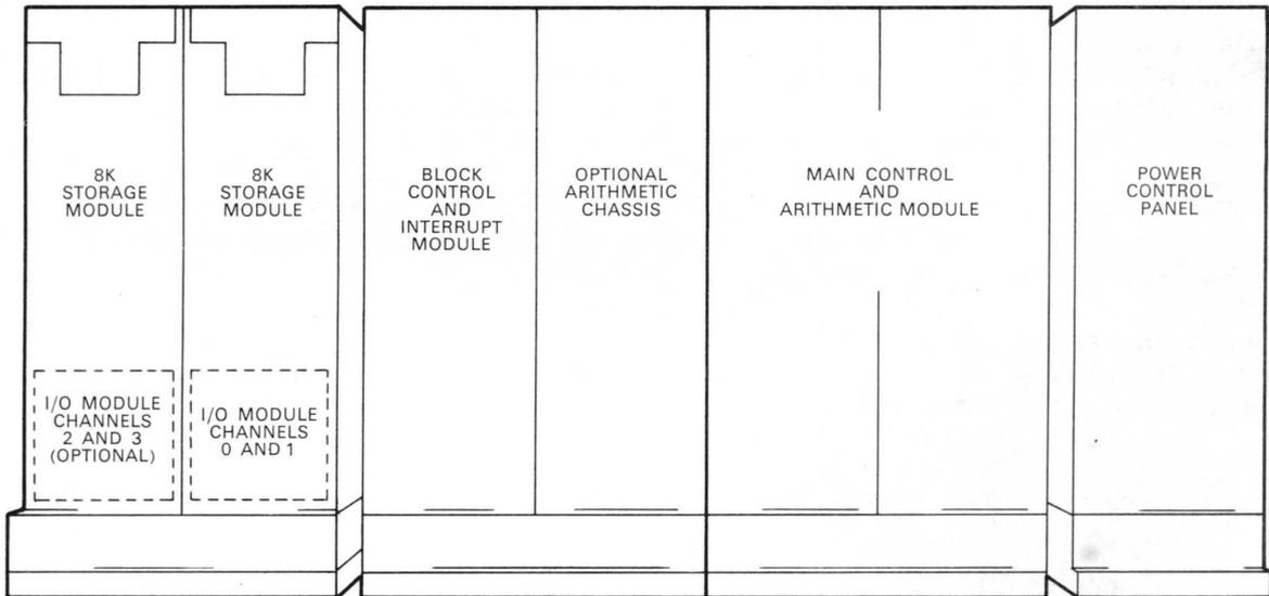
Figure 1-1. Typical 3200 Modular Configuration
