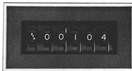
If the WRITE STO switch on the keyboard switch is depressed and data has been entered into the Communication register, the data is transferred to memory location 00104 when the Transfer switch is depressed.
