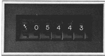
During the normal execution of a program, the computer stops when an RNI is attempted at memory location 05443. A jump to this location also causes the computer to stop. If the program references memory location 05443 for an operand, the computer ignores the Breakpoint switch.
