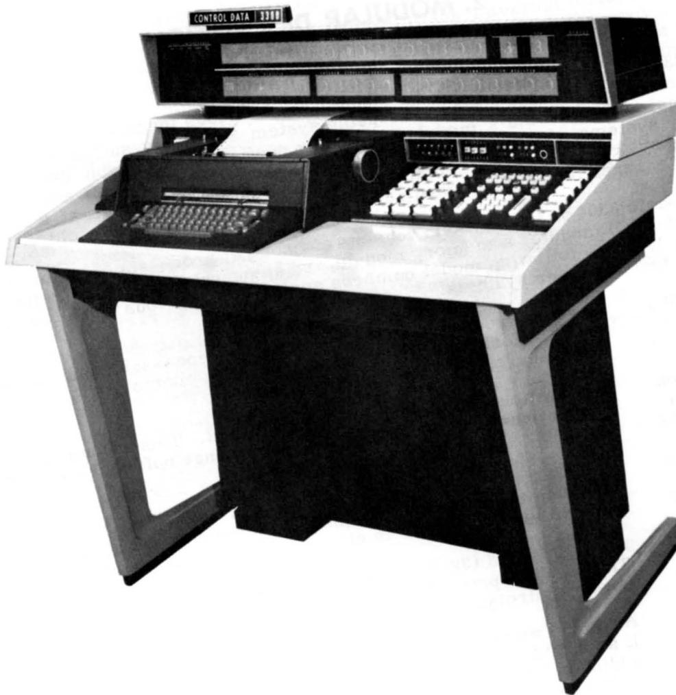
Figure 2-1. 3300 Computer System Console
