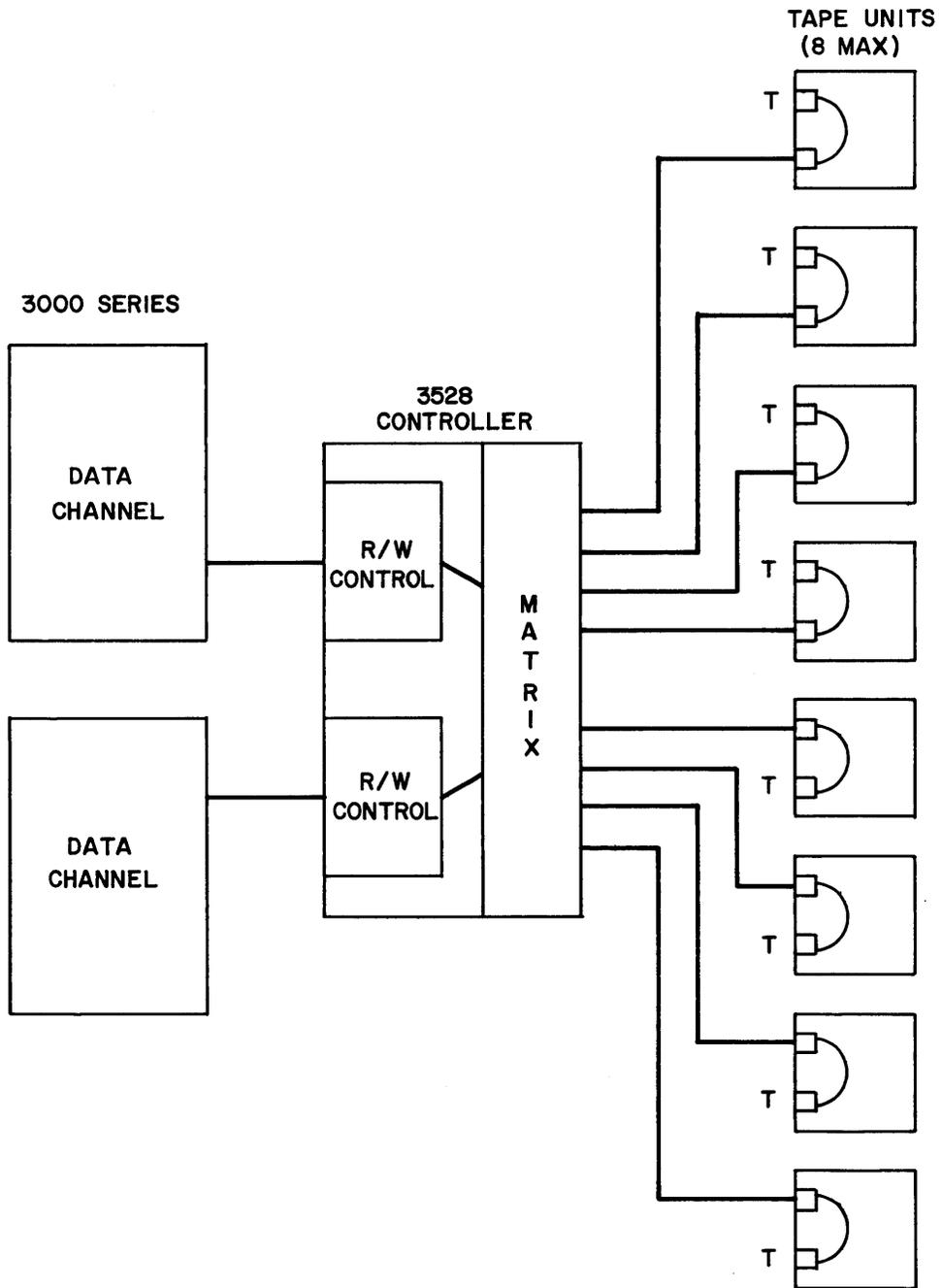
Figure 1-2. Typical Dual Channel Configuration
