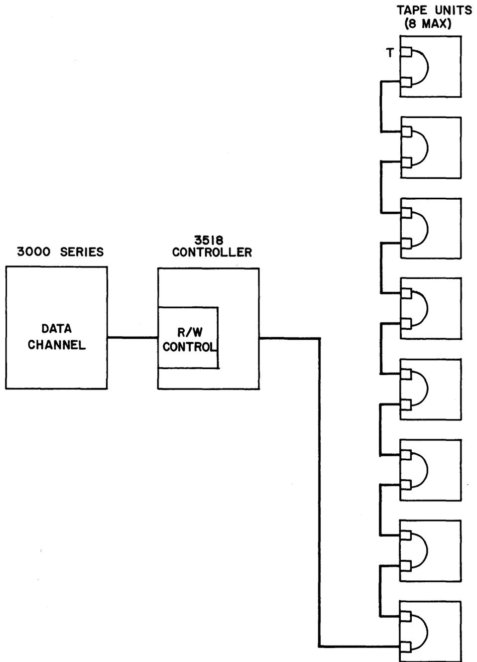
Figure 1-1. Typical Single Channel Configuration
