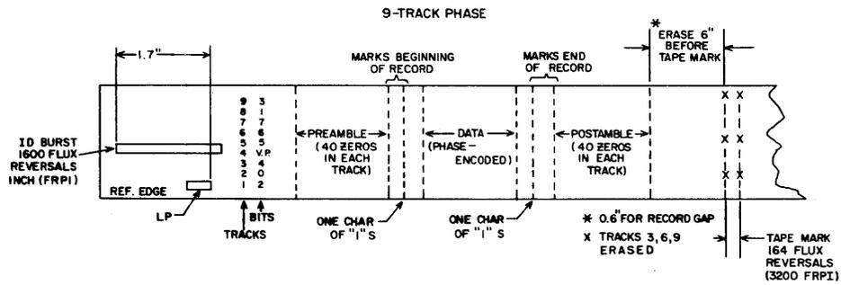
Figure 1-5. Phase Encoded Format
