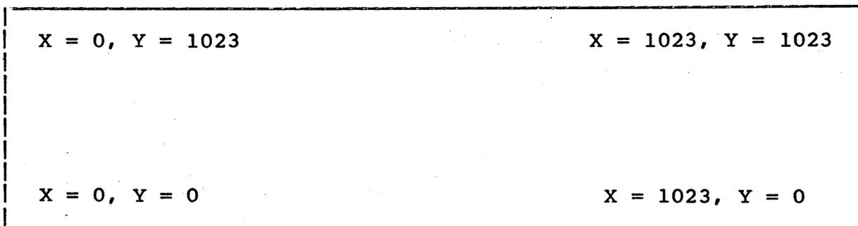
Figure 12-1. Display with Scaled Coordinates
