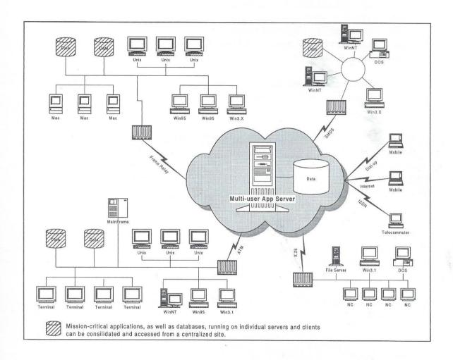
By consolidating the application on centralized servers and limiting the client workstation's job to display duties alone, the thin-client/server model has an assessment profile that differs sharply from the traditional application deployment approaches above.
