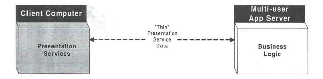
The thin-client/server model functions similarly to an N-tier client/server application that has been partitioned such that all business logic executes on intermediate application servers, leaving client workstations to display the user interface. However, they do differentiate: Thin-client/server architecture can centralize business logic of two-tier
