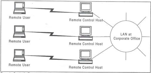
Remote Control: Remote control-based application deployments give remote users good performance since only screen updates are passed between the remote user's workstation and the local host computer. Unfortunately, the additional layer of hardware increases deployment costs and hinders scalability: Each new, concurrent remote user needs a local computer to control. MIS winds up managing local host computers in addition to local servers and remote users.
