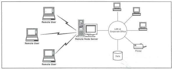
**Remote Node:** By effectively extending the local network to include remote users, remote node solutions make enterprise-wide application deployments easier to manage and scale. Remote clients are logically identical to their local counterparts, and applications run on local and remote machines in the same manner. Application performance, on the other hand, is stifled by comparatively low-bandwidth WAN and dial-up connections.
