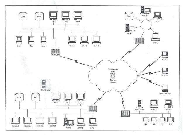
MIS rarely has the luxury of deploying mission-critical applications in a homogeneous environment, let alone from a centralized location. Instead, the enterprise network usually includes a widely-dispersed variety of servers, client workstations and operating systems. A variety of wide area connections connects remote office LANs throughout the nation or the world. The user base can include from dozens to thousands of local, remote, mobile, telecommuting users.
