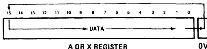
Figure 3-22. Rotate Right
