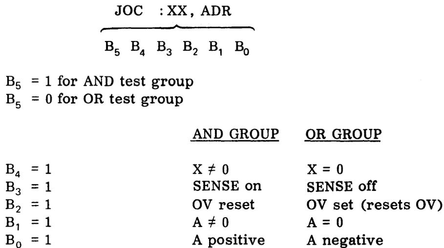
Figure 3-14. JOC Microcode Bit Functions
