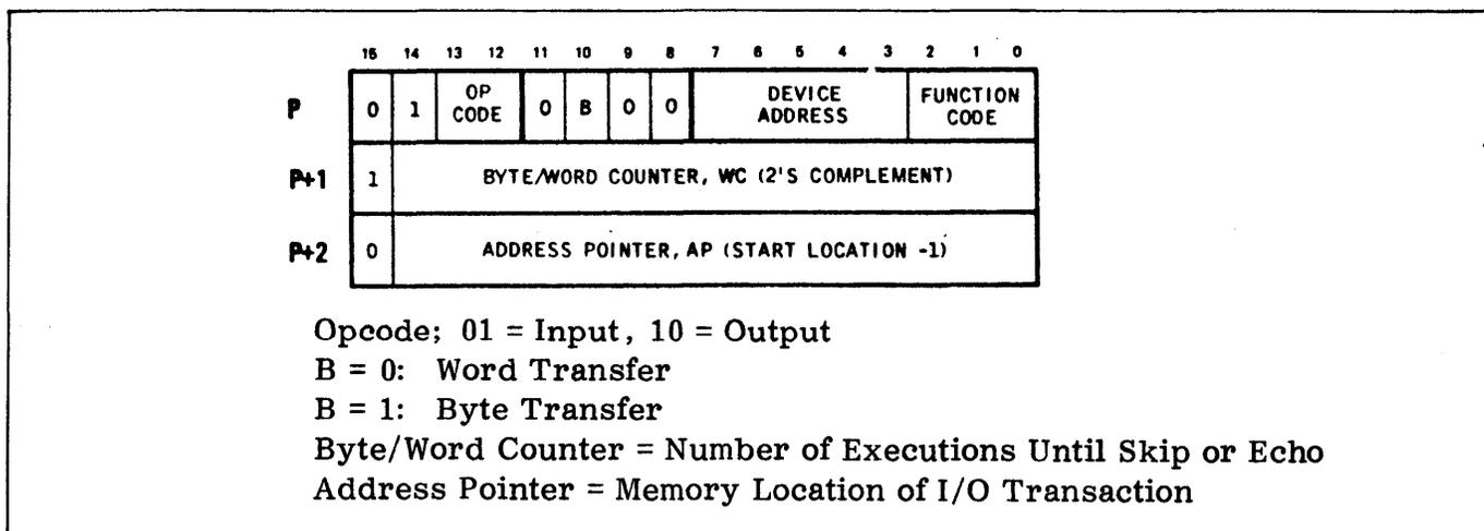
Figure D-10 Automatic Input/Output Instruction Machine Code Format
