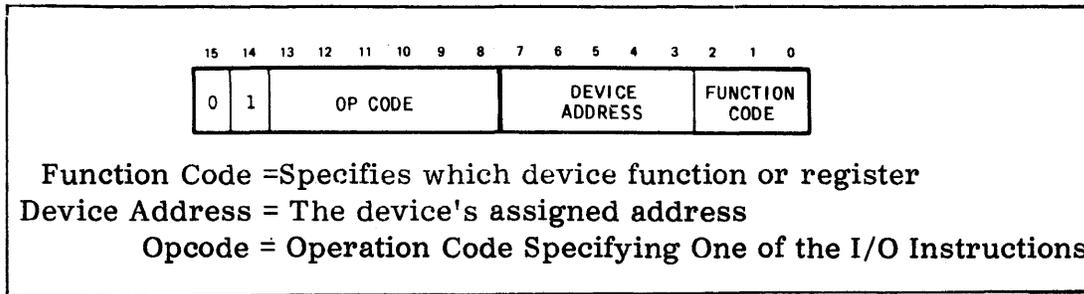
Figure D-9. Input/Output Instruction Machine Code Format
