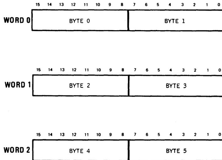
Figure 1-4. Data in Memory, Two Bytes Per Word
