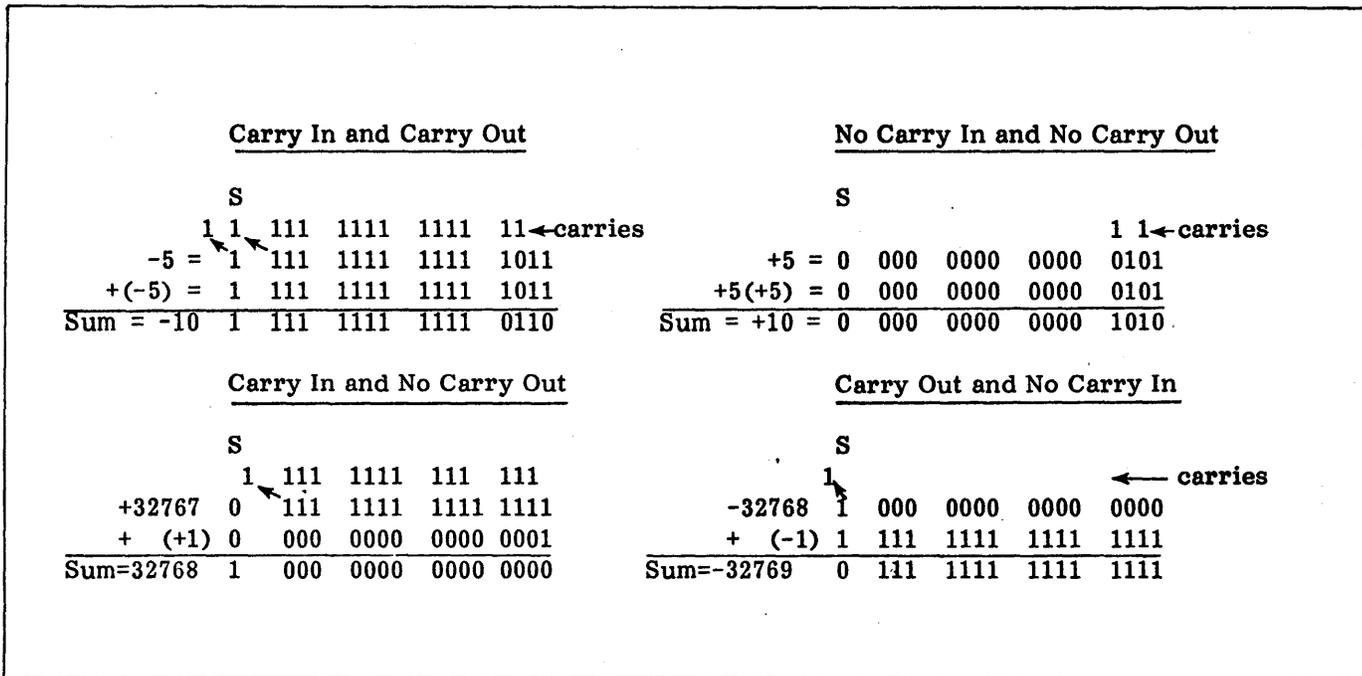
Figure 3-3. Arithmetic Overflow.
