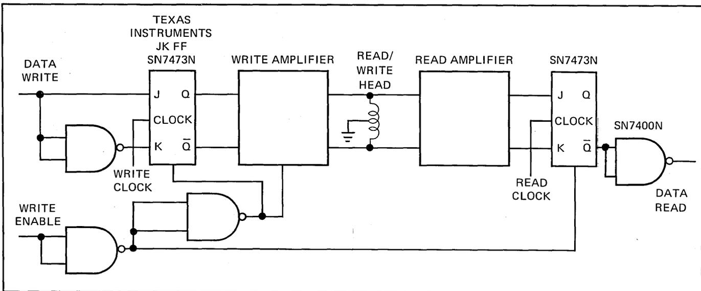
Figure 2-1 Read/Write Module
