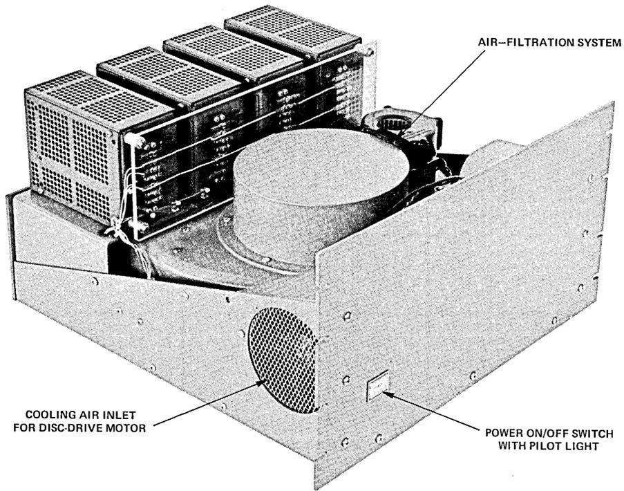
Figure 2-4 FPD Disc Memory System, Front View
