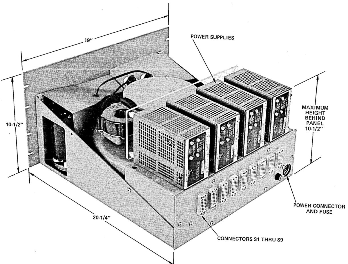
Figure 2-5 FPD Disc Memory System, Rear View
