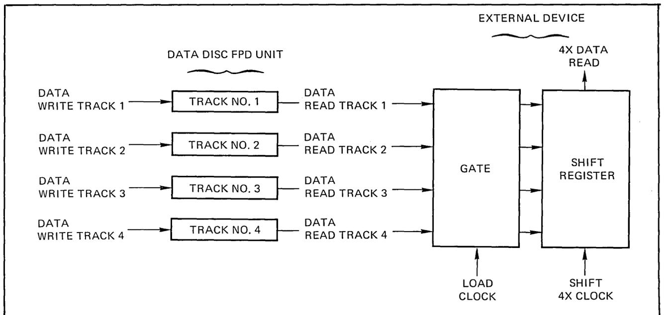
Figure 2-3 Four Tracks Read in Parallel and Serialized at a 4X Rate
