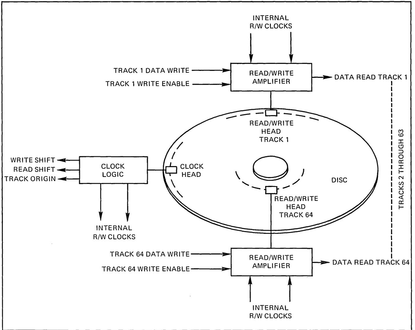
Figure 2-2 FPD Disc Memory System Block Diagram
