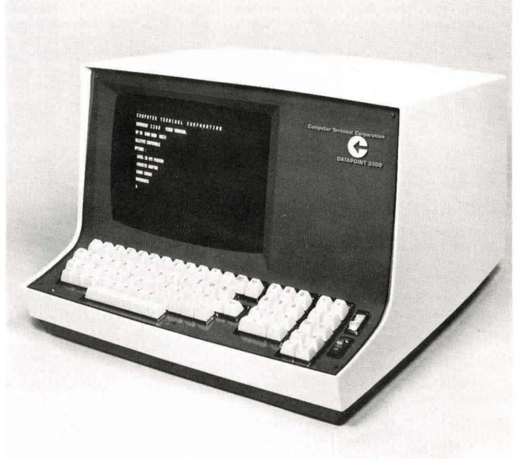
in a single glance and where necessary to make modifications and revisions. Program debugging is greatly simplified. With the 3300, the remote computer becomes a much more flexible aid to human thought processes. Data transmission rates of up to 2400 bits per second are available on the Datapoint 3300.
