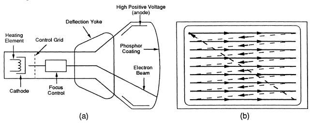
(a) The CRT produces images by generating a beam of electrons and focusing it onto a phosphorous-coated screen, which fluoresces or emits light at the point of contact. (b) The beam sweeps the screen from top to bottom and left to right in a pattern called a raster scan.
