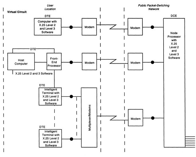
Signifies an interface that must conform to X.25 Level 2, Physical Interface Standards.
