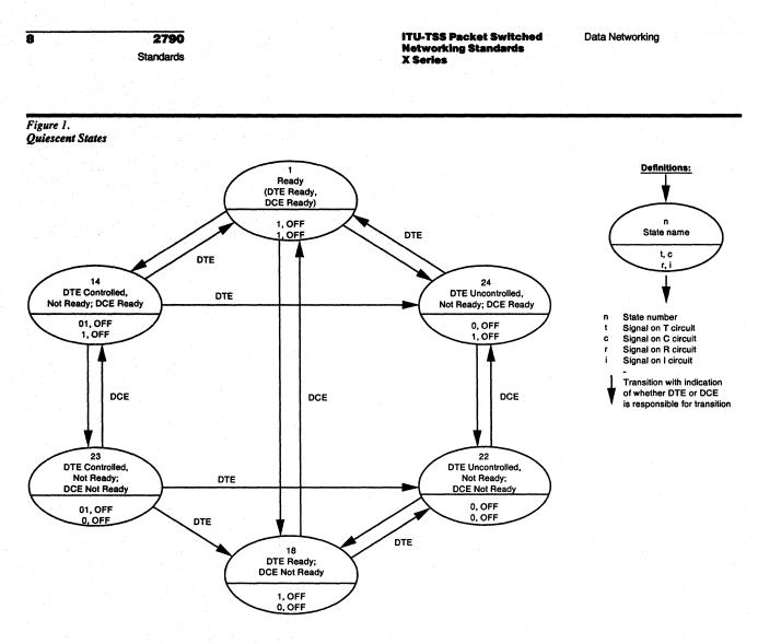
The above diagram indicates transitions that are allowed in X.21 networks. Other transitions are possible and may be allowed in some networks. See Table 3 for a listing of possible transitions.
