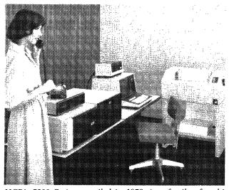
NCR's 7500 Series, unveiled in 1978, is a family of multipurpose intelligent terminal systems. Three model configurations are available, including the 7530, shown here. Applications range from a remote batch workstation to a desktop small business computer.
