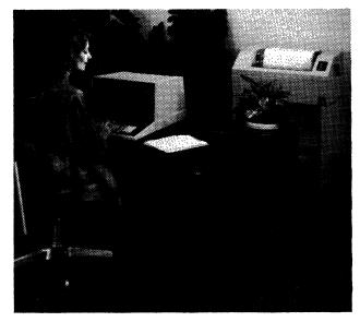
The NCR 7520 Small Business System package offers data and information processing capabilities to the small business user. System components include a CRT/processor, keyboard, dualdrive flexible disk module, Model 6440 matrix printer, and the BASIC +6 software interpreter.
