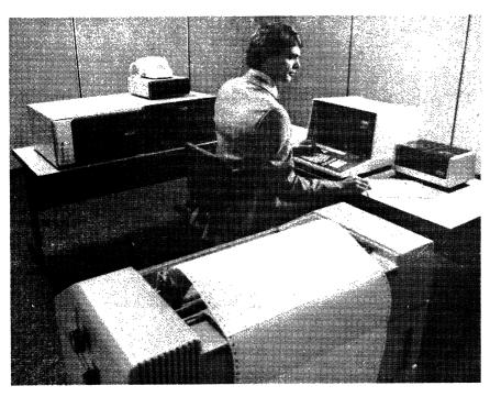
NCR's 7530, the most sophisticated member of the 7500 Series, can support a wide variety of peripherals, including a 50- to 125-lpm matrix printer (foreground); a ½-inch magnetic tape drive, dual diskette drive, and bisynchronous communications adapter (left of operator); and a magnetic tape cassette drive (right of operator).
