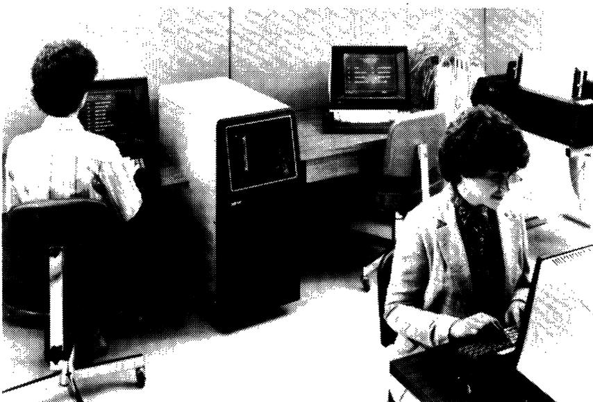
*Northern Telecom's Model 585 is a medium cluster DDP/WP system. The 585 processor has a main memory capacity of up to 512K bytes; total disk storage capacity is 342 megabytes. The 585 can support up to 16 displays or printers, and is compatible with previous Northern Telecom DDP systems, including the 405, 435, and 445.*
