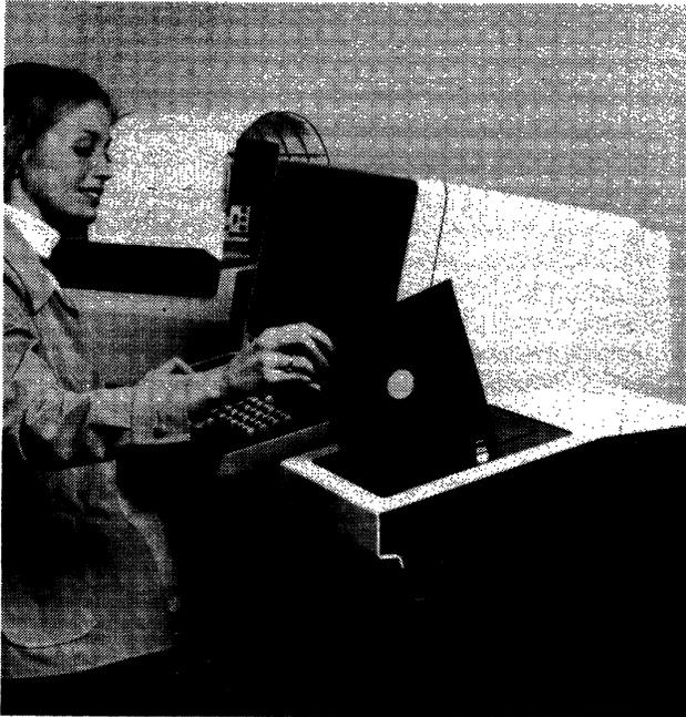
*This stand-alone Sycor 250 terminal consists of a CRT display, keyboard, printer, and dual diskette unit (foreground). In cluster configurations, a Sycor 250 System can include any mix of up to 32 keyboard/display units and printers.*
