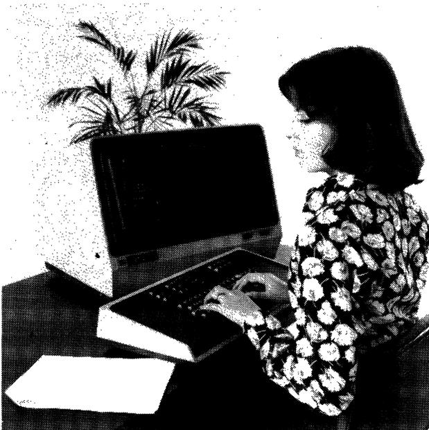
*The Sycor 350 Intelligent Terminal is a more powerful and flexible version of the earlier 340. Introduced in June 1975, the stand-alone terminal contains integral dual diskette drives (to the right of the display screen) in place of the 340's cassette tape drives.*
