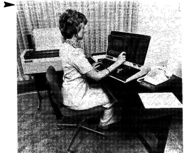
*The Sycor 350 Intelligent Terminal is a more powerful and flexible version of the earlier 340. Introduced in June 1975, the stand-alone terminal contains integral dual diskette drives (to the right of the display screen) in place of the 340's cassette tape drives. An additional dual-diskette drive is optional. Sycor also offers a packaged version of the 350, the 357, which includes a communication interface and printer.*
