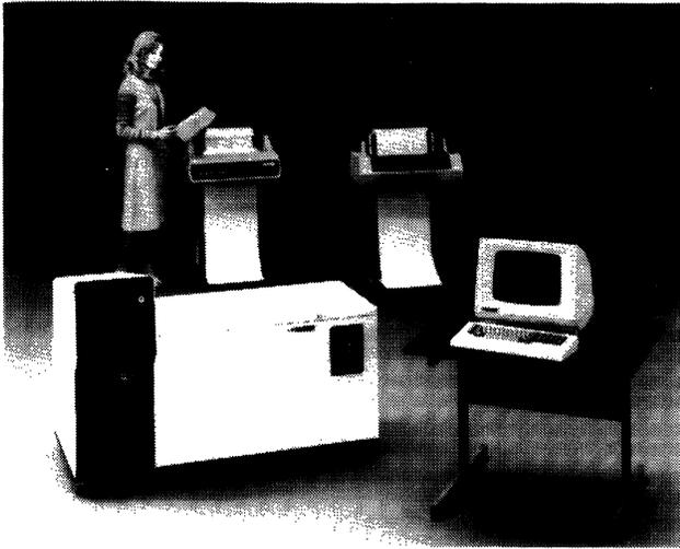
The Sycor 445 controller (left foreground) with fixed-disk extension cabinet is surrounded by components common to both Sycor 405 and 445 terminal systems. These components include (from left) the 300-lpm Strider (GE TermiNet 340) printer, bi-directional Sprinter matrix printer, and 15-inch display station.
