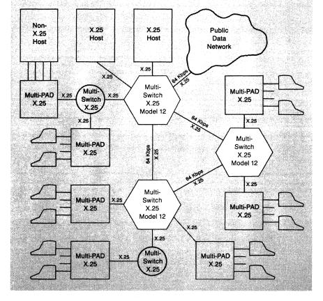
Figure 1. The Multi-PAD X.25 is often used with Dynapac's Multi-Switch X.25, which routes data from one X.25 trunk to another. Pictured here is an example of a large private data network incorporating Multi-Switch Model 12s and a number of Multi-PAD X.25s linking asynchronous terminals, hosts, and a public data network.
