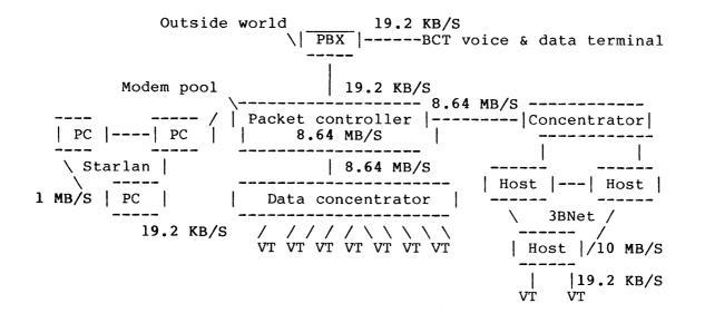
Note the BCT (Business Communications Terminal) voice and data terminal in the above display. Even though the terminal is a voice AND data terminal, which can impress a novice buyer, voice and data messages are not necessarily integrated. Your customer needs to understand the difference between physical integration and functional integration. Your customer also needs to understand that this is not what is meant by ISDN (integrated voice and data) today.
