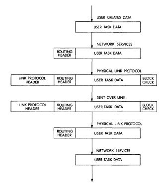
Figure 3-3 Data Flow Through the System
