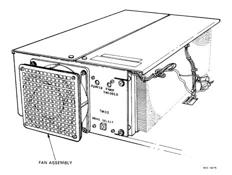
Figure 1-5 TM03 Front Panel
