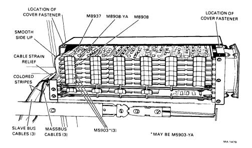
Figure 3-1 TM03 Formatter with Cover Removed
