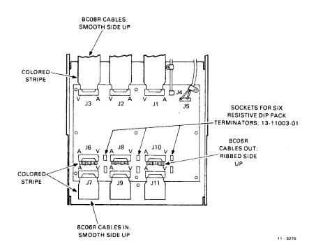
Figure 3-7 Cable Orientation on M8928 MTA Module
