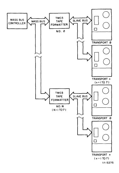
Figure 1-1 TM03 Tape Transport System Configuration
