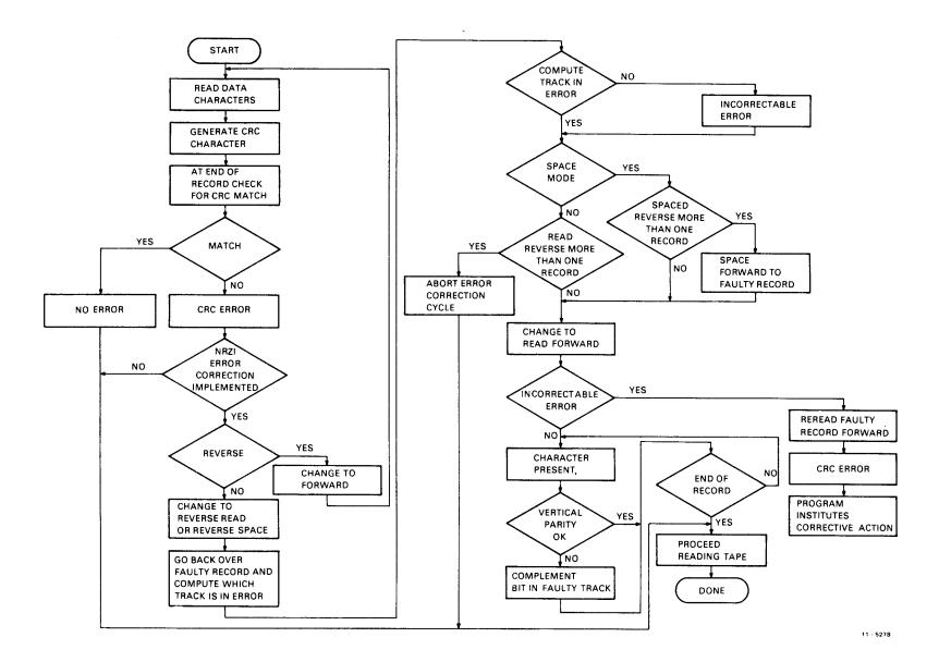
Figure 2-10 NRZI Error Correction Flow Diagram
