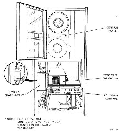
Figure 1-4 TM03 with TU77 Tape Transport in H9500 Corporate Cabinet
