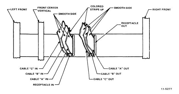
Figure 3-6 Internal Cabling to Massbus Connector Panel in H9500 Corporate Cabinet
