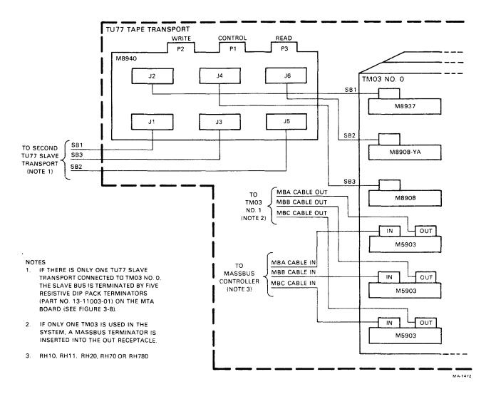
Figure 3-4 TM03 Cabling to an M8940 MTA Adapter Board in a TU77 Transport in an H9500 Corporate Cabinet
