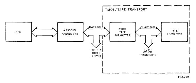
Figure 1-6 TM03 in a System Configuration
