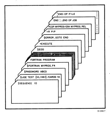
Batch puts the following commands into the control file as a result of the cards you entered.
