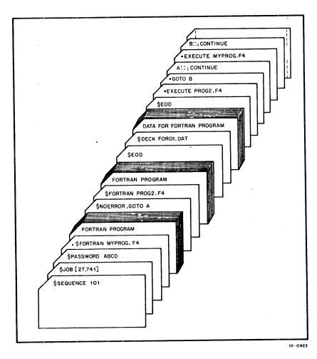
Batch reads the cards and puts the following commands into the control file.
