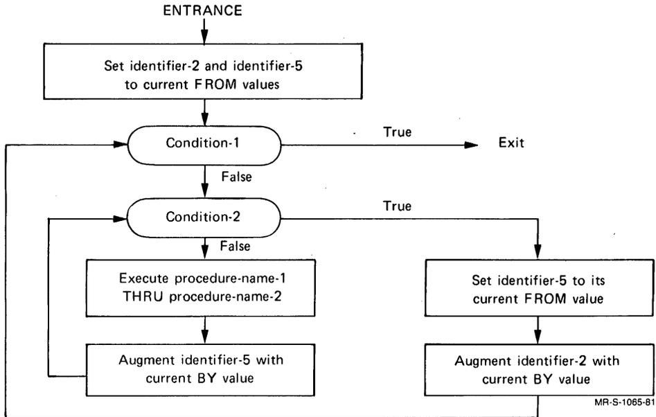
The following flow chart illustrates the logic of the PERFORM cycle when three identifiers are varied.
