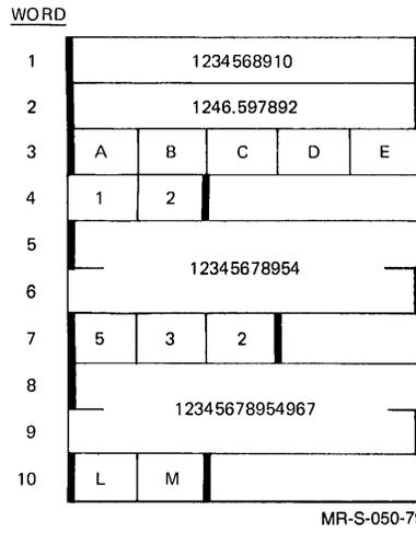
Figure 8-21 COBOL Standard Binary and ASCII Mixed-Mode Binary
