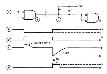
Figure B-9 Positive Edge Triggered One-Shot (used only by memory logic)
