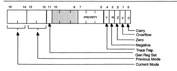
Bits 15 or 14 indicate the current processor mode: user mode (11), supervisor mode (01), or kernel mode (00). Bits 13 and 12 indicate the previous mode, that is, the mode the machine as in (user, supervisor, or kernel) prior to the last interrupt or trap.
