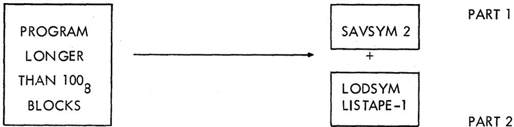
A SAVSYM 2 during the assembly of PART 1 will save all the symbols from PART 1. The LODSYM at the start of PART 2 loads in the saved symbol table, thus putting all the symbols from PART 1 and PART 2 into a common symbol table. For DIAL-MS, LISTAPE with a negative argument can be used to preserve the bit map from the assembly of PART 1.
