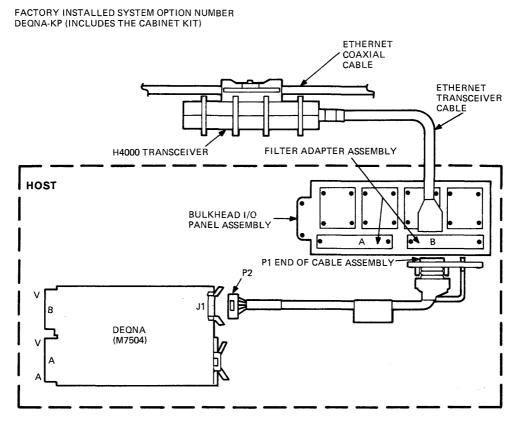
Figure 1-4 DEQNA to ETHERNET Connection
