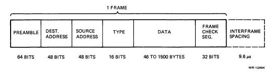
Figure 1-3 ETHERNET Packet (Frame) Format
