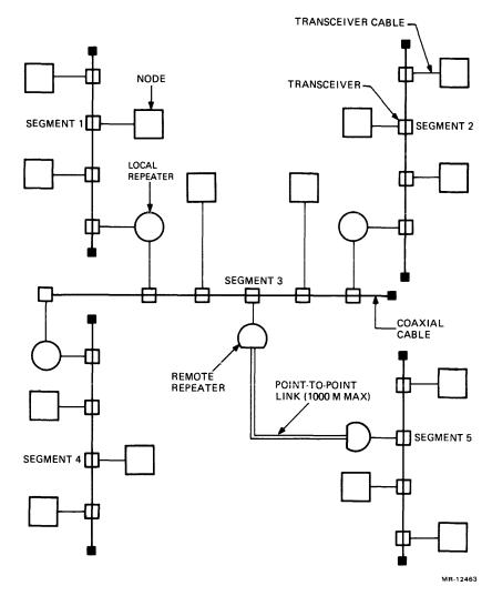
Figure 1-1 Large-Scale ETHERNET Configuration
