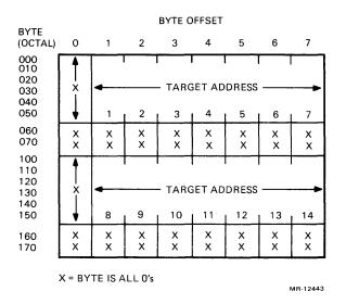
Figure 4-3 Target Address Set-Up
