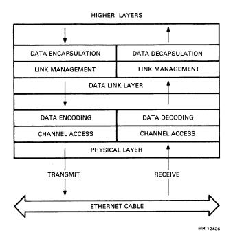
Figure 1-2 ETHERNET Layer Functions
