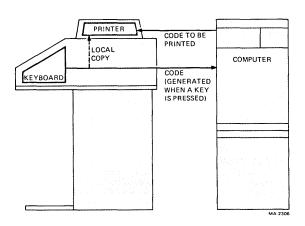
information (a code) to a computer. Second, it is a printer; information is sent from the computer to the printing portion of the LA120. However, you can set up your system to send information from the keyboard to the printer and computer at the same time.
