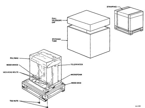
Figure 2-2 Unpacking/Packing
