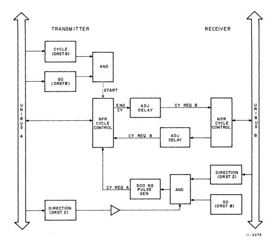
Figure C-4 NPR Interlocking Control Block Diagram
