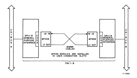
Figure C-1 Block Diagram of PDP-11 DMA Interprocessor Channel
