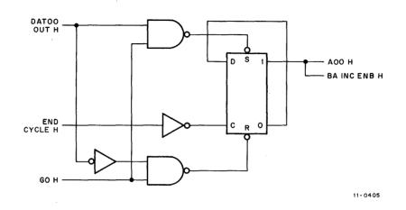
Figure 6-3 Byte Addressing, Additional Function (Compare with Figure 6-2.)
