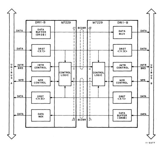
Figure C-2 DMA Interprocessor Channel Functional Block Diagram
