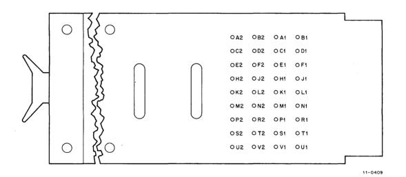
Figure B-1 M957 Cable Connector Pinning Detail
