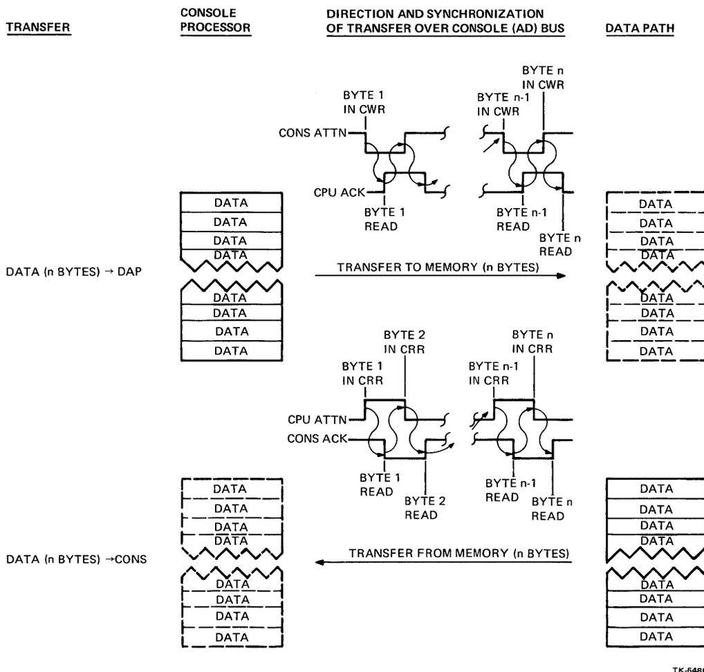
Figure 2-22 Communications Over Console Bus in Console Mode
