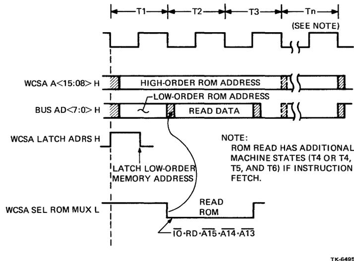
Figure 2-17 8085A ROM Read Operation Timing Diagram
