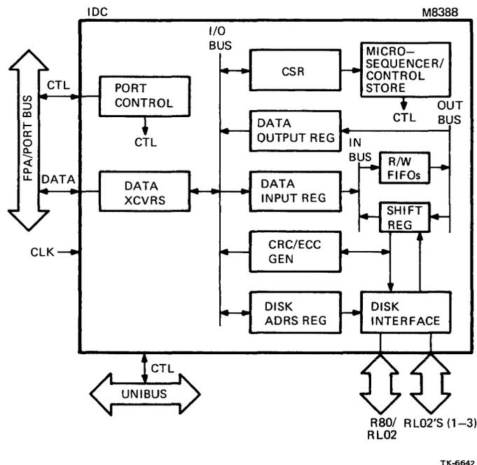
Figure 1-4 Integrated Disk Controller
