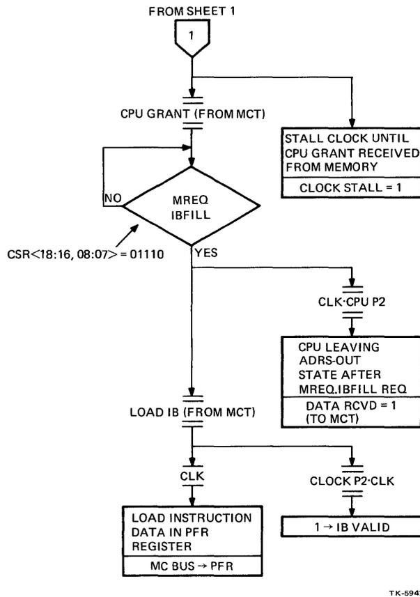
Figure 6-22 MEM REQ Microinstruction Flow Diagram (Sheet 2 of 2)
