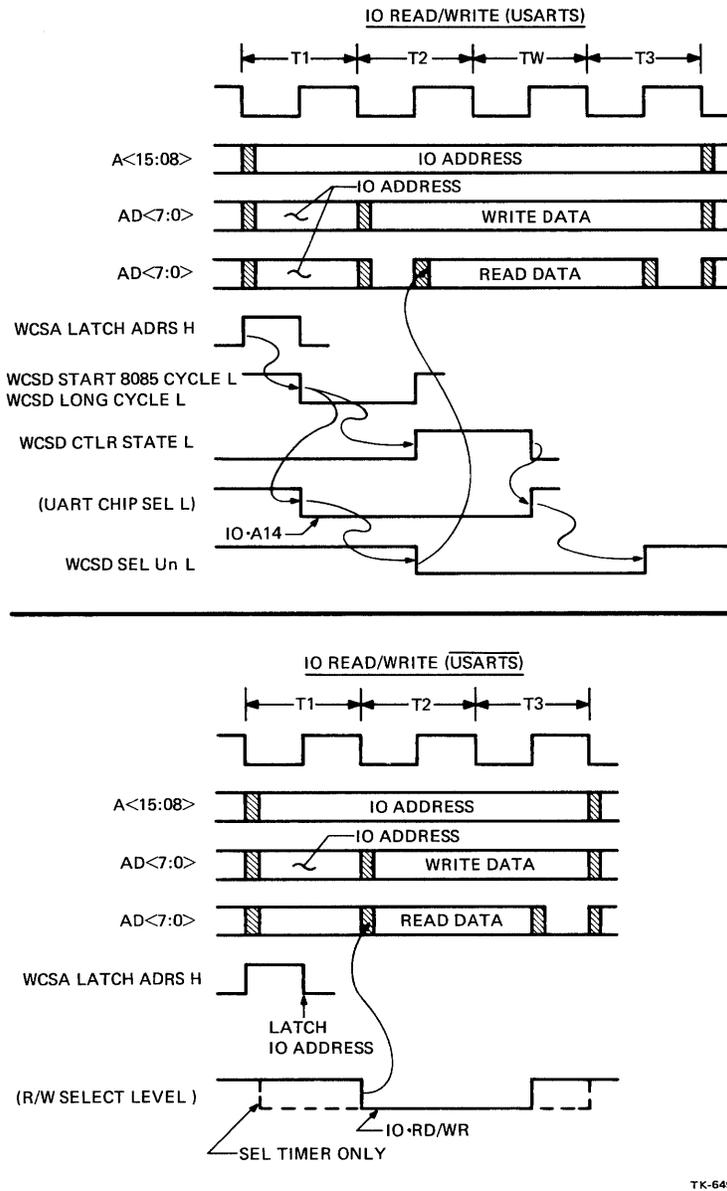
Figure 2-21 8085A I/O Read/Write Operations Timing Diagram
