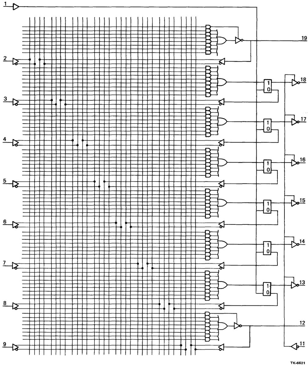
Figure A-9 16R6 PAL Device Logic Diagram
