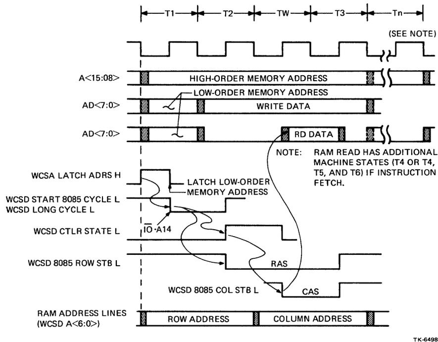
Figure 2-18 8085A RAM Read/Write Operations Timing Diagram
