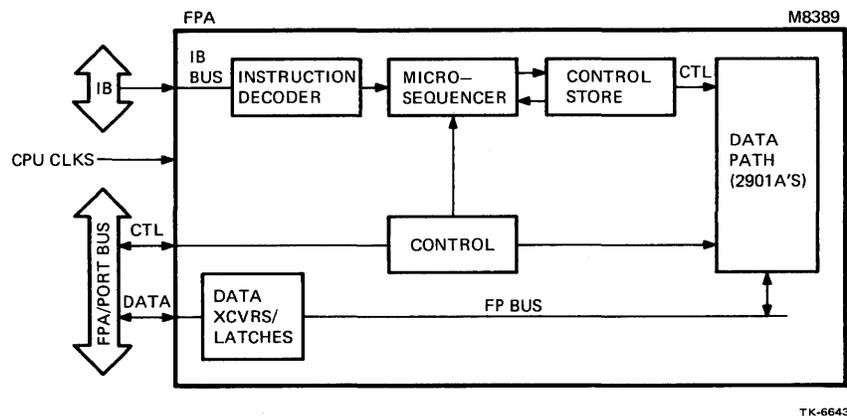
Figure 1-3 Floating-Point Accelerator
