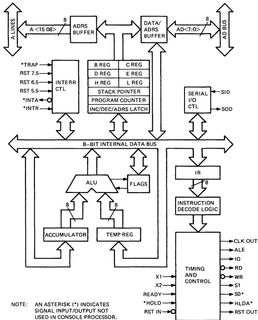
Figure 2-2 8085A Microprocessor
