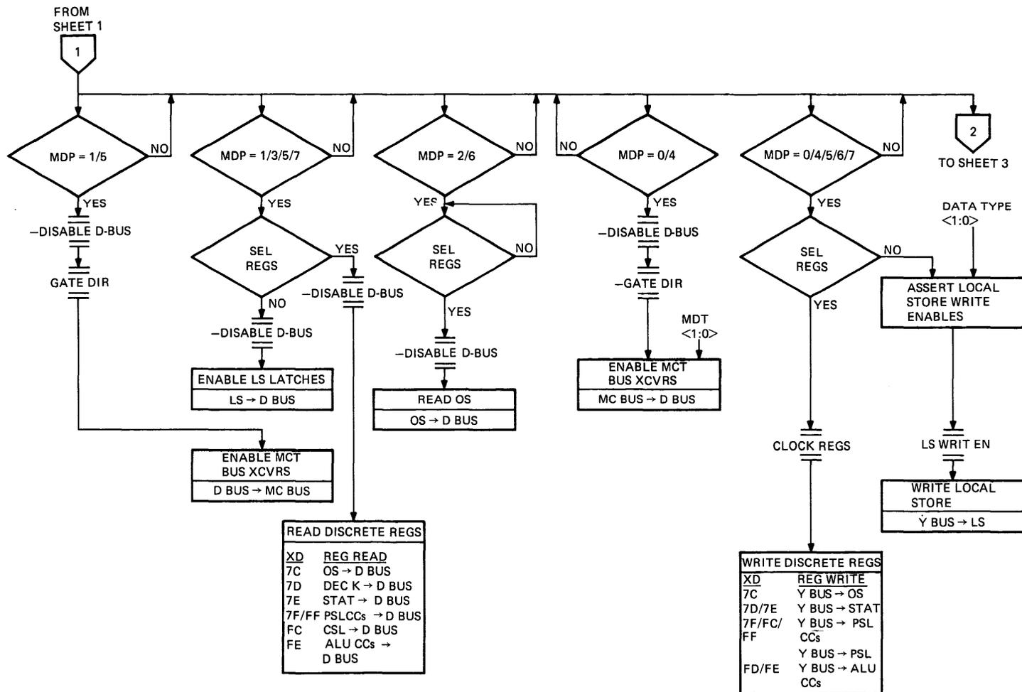
Figure 6-23 MOVE Microinstruction Flow Diagram (Sheet 2 of 3)
