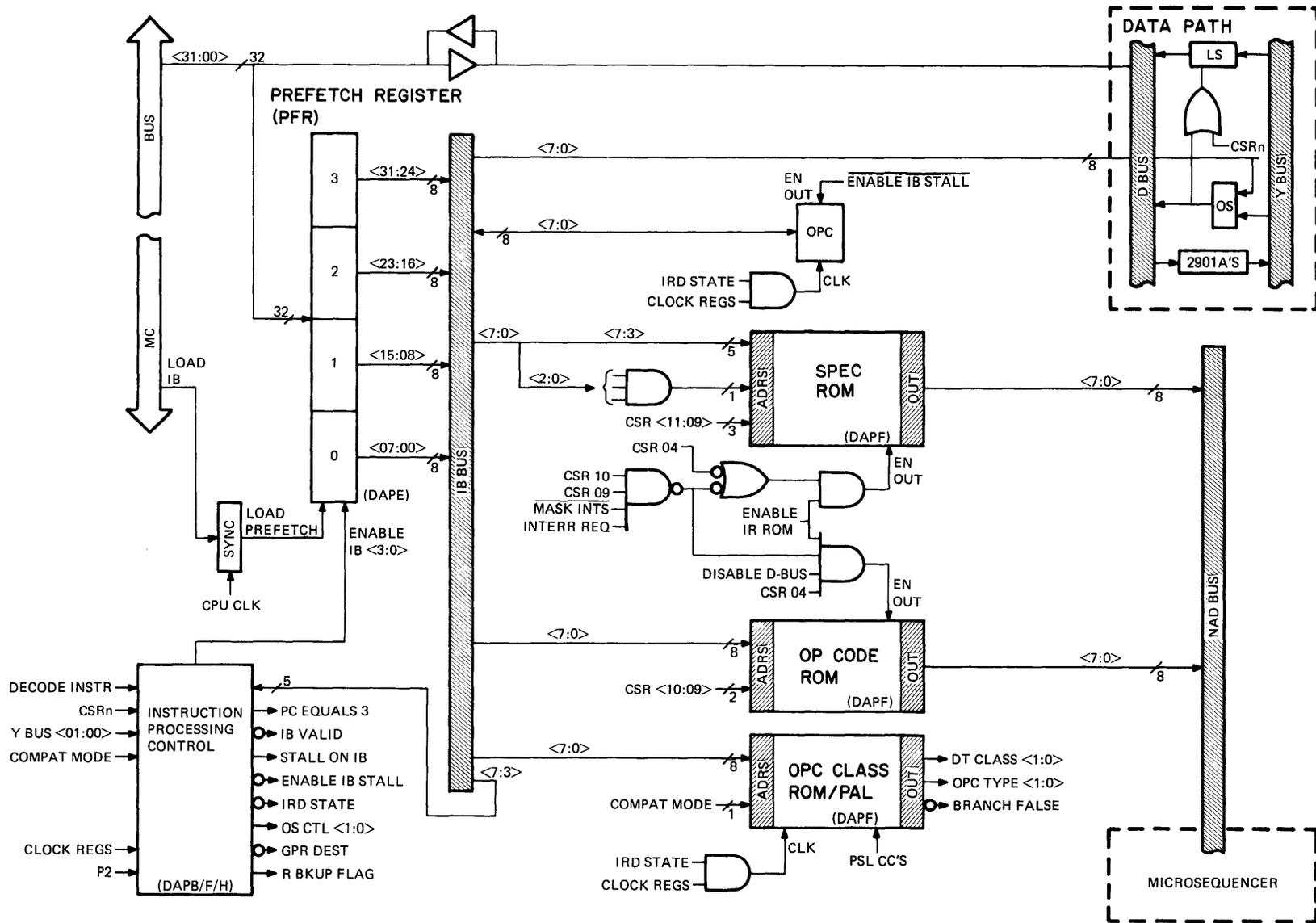
Figure 5-1 Instruction Processing Hardware Block Diagram
