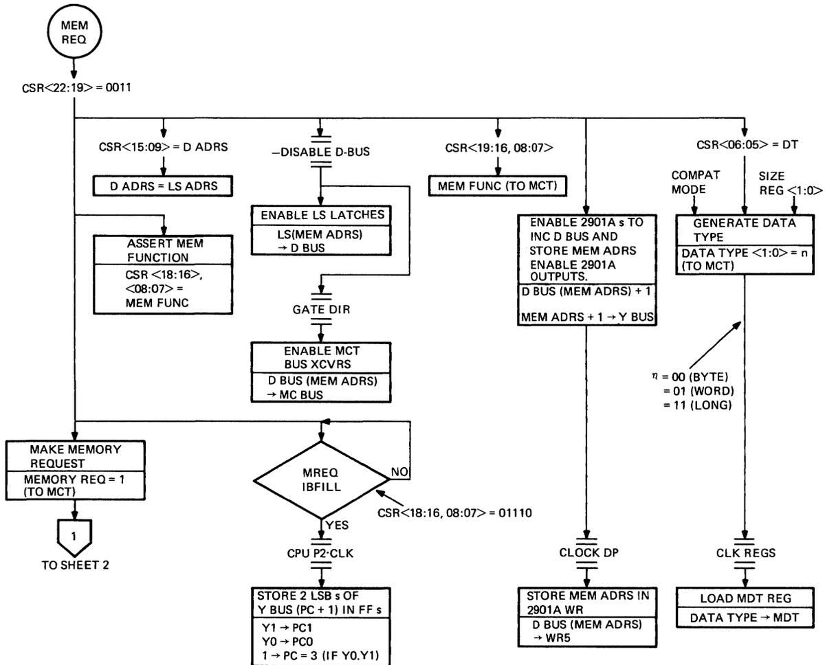
Figure 6-22 MEM REQ Microinstruction Flow Diagram (Sheet 1 of 2)
