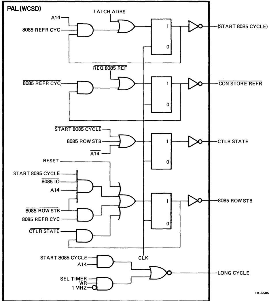
Figure 2-16 RAM/USART Control Logic (Sheet 1 of 3)
