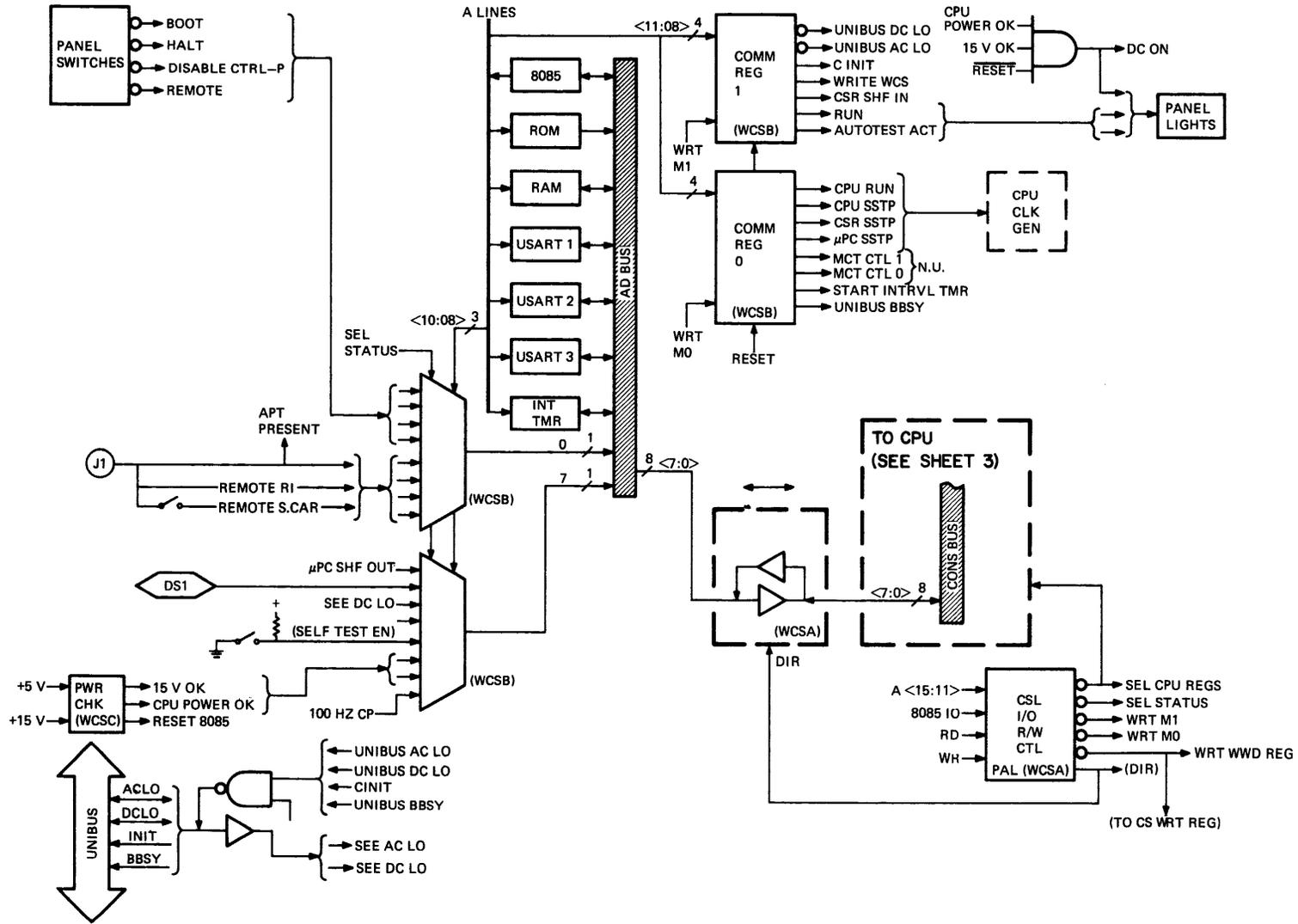
Figure 2-1 8085A Console Processor (Sheet 2 of 3)
