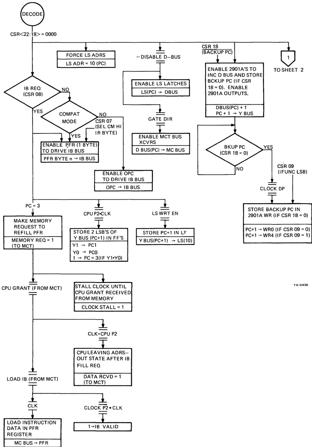
Figure 5-13 DECODE Microinstruction Flow Diagram (Sheet 1 of 2)
