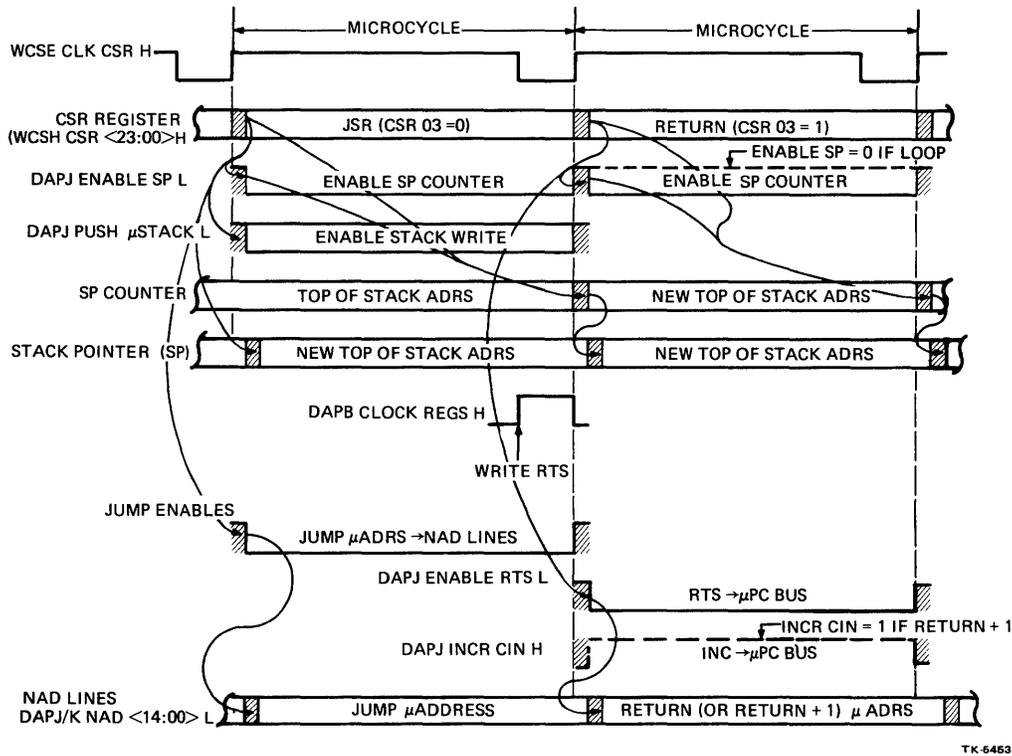
Figure 4-12 JSR/Return Timing Diagram
