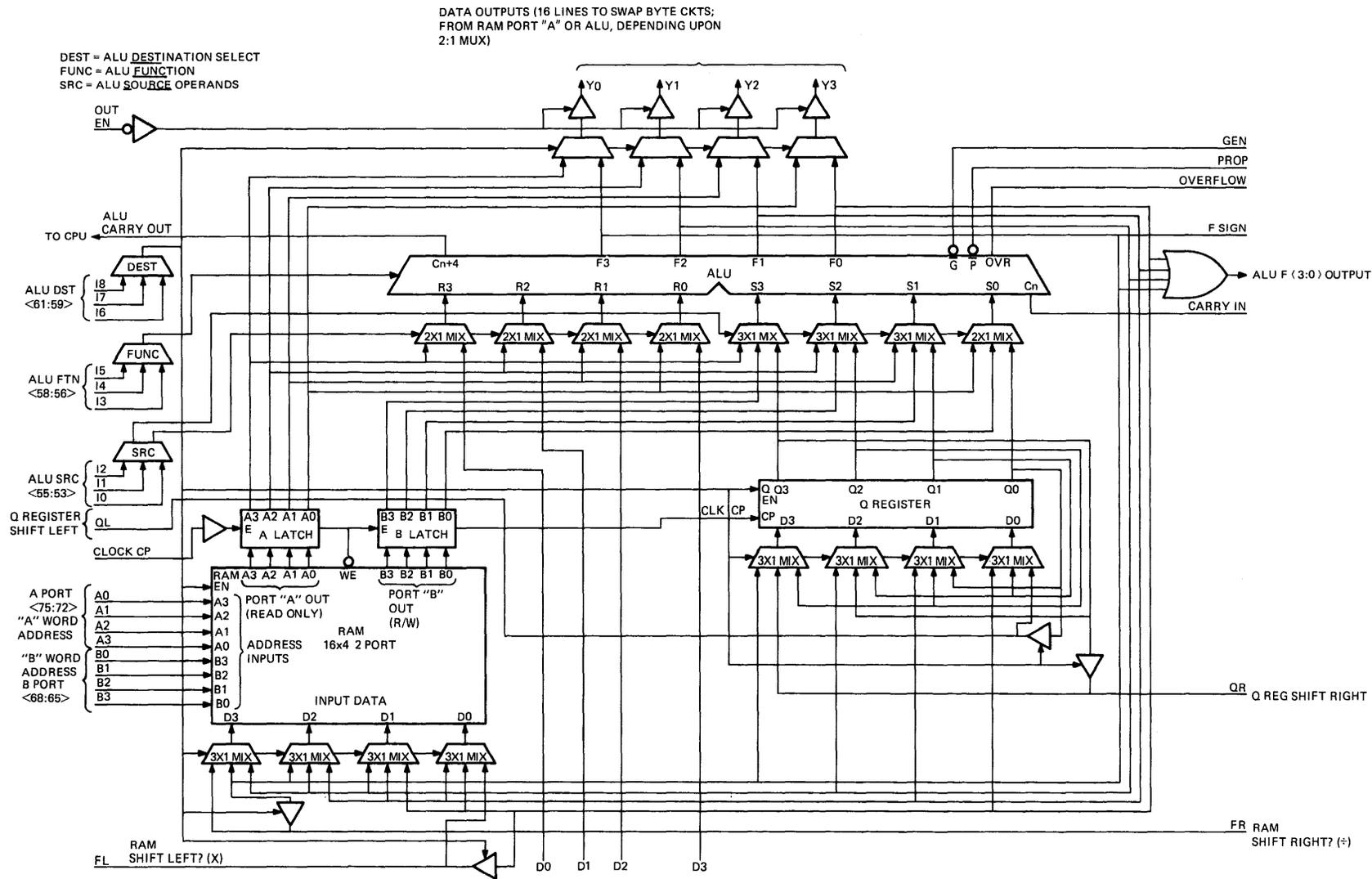
Figure 6-4 2901A Microprocessor Slice – Detailed Block Diagram
