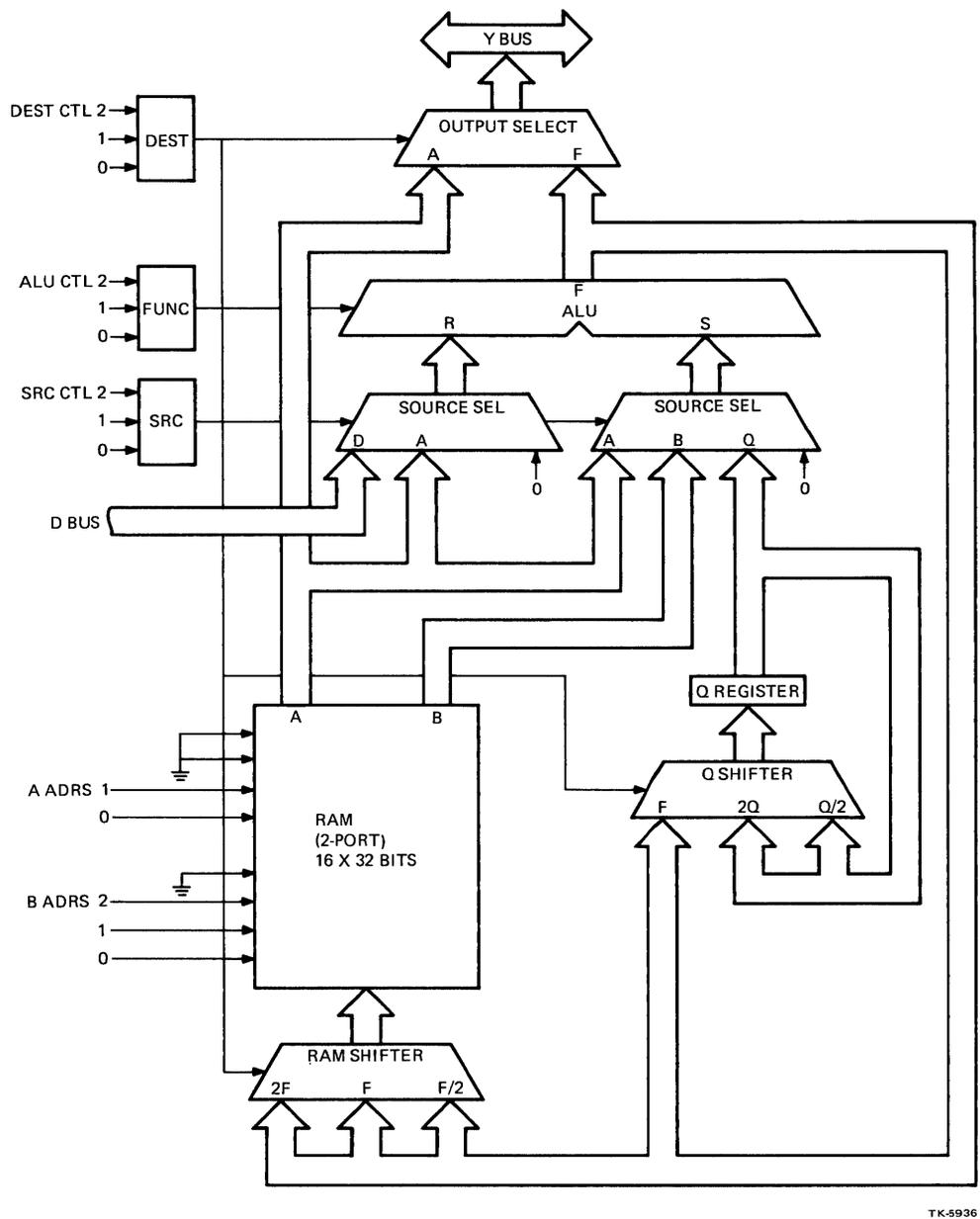
Figure 6-5 Data Processor (Eight 2901As) Simplified Block Diagram
