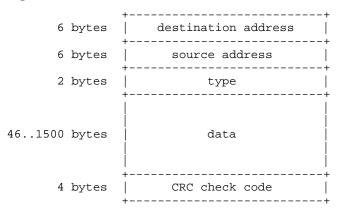
The minimum size of a packet is 64 bytes, which implies a minimum data length of 46 bytes. Packets shorter than this are called "runt packets" and are treated as erroneous when received by the network controller.
