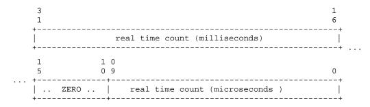
Note 1 : the actual count source for the high resolution timer is 1.017  $\mu s,$  thus the maximum count will overflow every 1.042 milliseconds.
