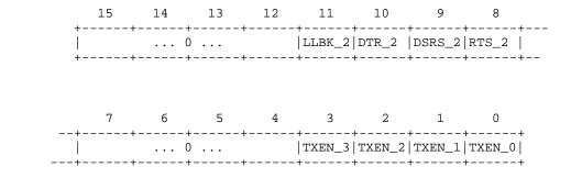
Figure 11–4: Serial Line Transmitter Control Register (SER\_TCR)
