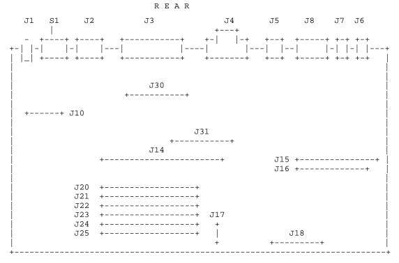
Figure 16–1: System Board connector Placement
